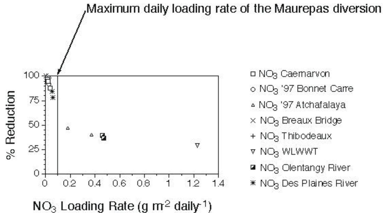
**Figure 3.** Daily nitrate loading rate versus removal efficiency for various river diversions and wetland wastewater treatment systems. Data sources: Caernarvon, Lane et al. 1999; Bonnet Carre, Lane et al. 2001a; Atchafalaya, Lane et al. 2001b; Breaux Bridge, Breaux and Day 1994 and Blahnik and Day 2000; Thibodeaux, Breaux and Day 1994 and Zhang et al. 2000; WLWWT, Olentangy River, Spieles and Mitsch 2000, Des Plaines River, Hey et al, 1994.
