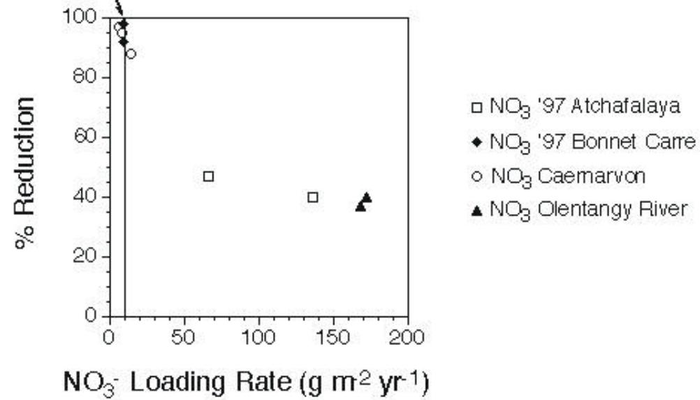
**Figure 2. Yearly nitrate loading rate versus removal efficiency for various river diversions.**
