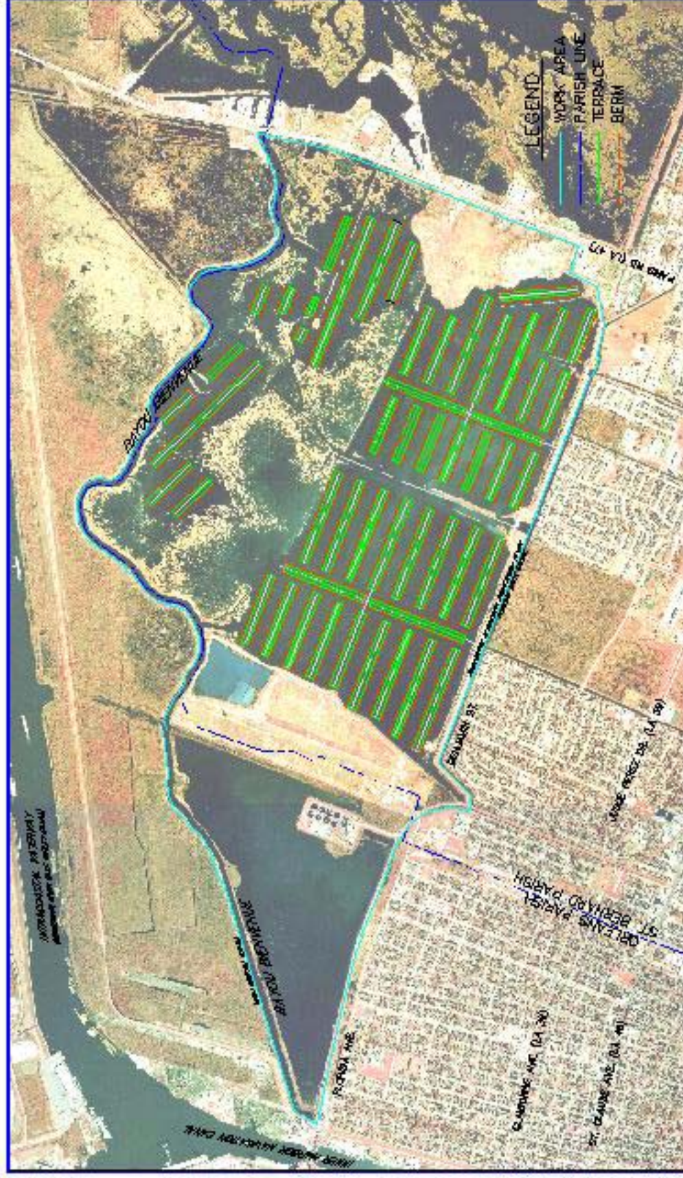
FIGURE 4 - AERIAL LAYOUT SHOWING TERRACE ORIENTATION 1 APPROXIMATELY 30,000 LINEAR FEET OF TERRACES SHOWN
