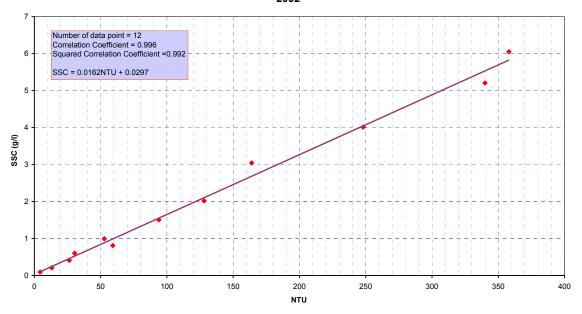
Figure 6. Calibration of near-bottom optical backscatter sensor (OBS) at Raccoon Island, Louisiana, 2002.
