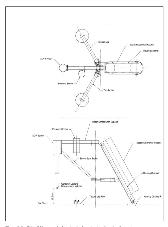
Figure 3. SonTek ADV sensor platform in planform (top) and section (bottom).
