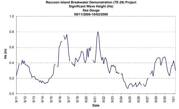
Figure 9. Time series of significant wave height (Hs) at deployment #4 (D4)
