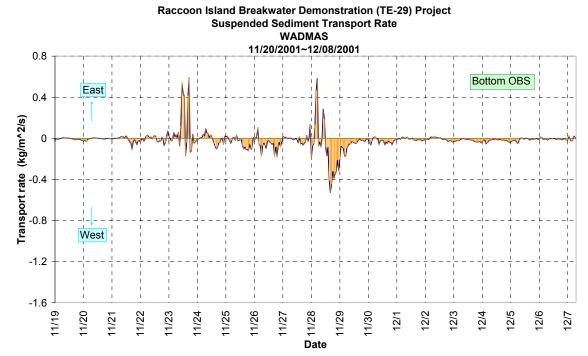
Figure 34. Time series of bottom long shore suspended sediment transport rate at D6.
