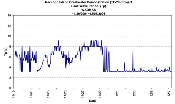
Figure 17. Peak wave period (Tp) at deployment #6 (D6).
