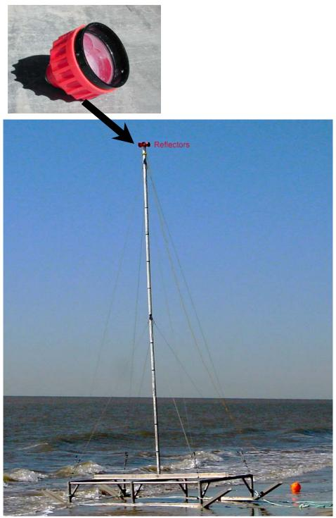
Figure 7. Sled used in bathymetric surveys in the Raccoon Island area. Six reflectors were placed on top of the mast that stands on the sled. The height from the bottom to the reflectors is 6.6 m (21.65 ft).
