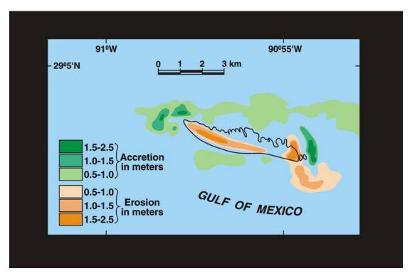
Figure 72. Bathymetric comparison from the 1940s through 1980s modified from List (1994).
