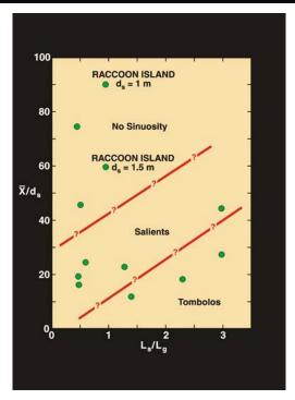
Figure 70. Upper, typical response of nearshore to breakwater construction. Middle, model of the response of Raccoon Island to breakwaters. Bottom, documented response of beaches to structures based on design criteria where X = distance offshore,  $d_s$  = depth at structure,  $L_s$  = structure length and  $L_g$  = gap width according to Pope and Dean, (1986).
