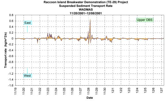
Figure 36. Time series of upper long shore suspended sediment transport rate at D6.
