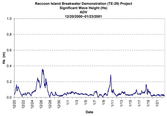
Figure 14. Significant wave height (Hs) at deployment #2 (D2).
