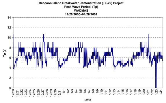
Figure 13. Peak wave period (Tp) at deployment #3 (D3).
