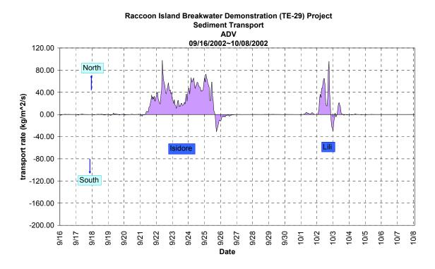
Figure 41. Time series of long shore suspended sediment transport rate at D7.
