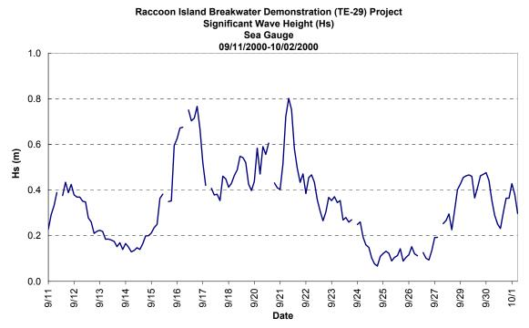
Figure 8. Time series of significant wave height (Hs) at deployment #1 (D1)
