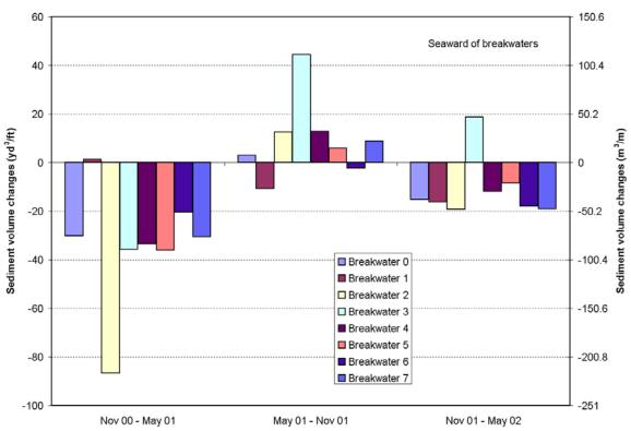
Figure 68. Sediment volume changes of the part in front of the breakwater of the eight survey lines through the breakwaters. Negative values represent erosion, while positive values represent deposition.
