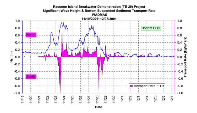
Figure 37. Time series of significant wave height and cross-shore suspended sediment transport rate at D6.
