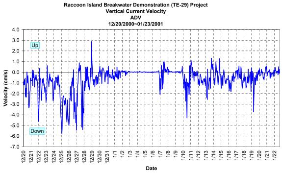
Figure 20. Time series of mean vertical current at D2.
