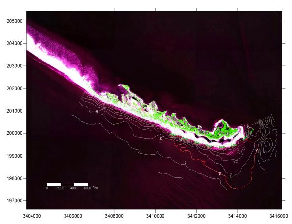
Figure 50. Image of Raccoon Island showing shoal fronting the breakwaters delineated by the 1.83 m (6 ft) isobath. Bathymetry is based on a May 2002 survey (relative to NAVD88).
