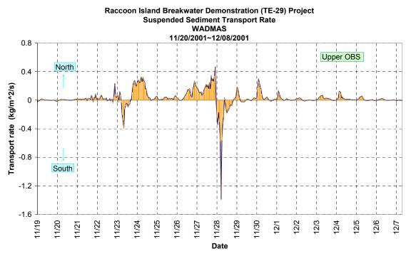
Figure 35. Time series of upper cross shore suspended sediment transport rate at D6.
