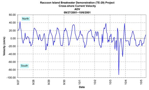
Figure 23. Time series of mean cross-shore current at D5.
