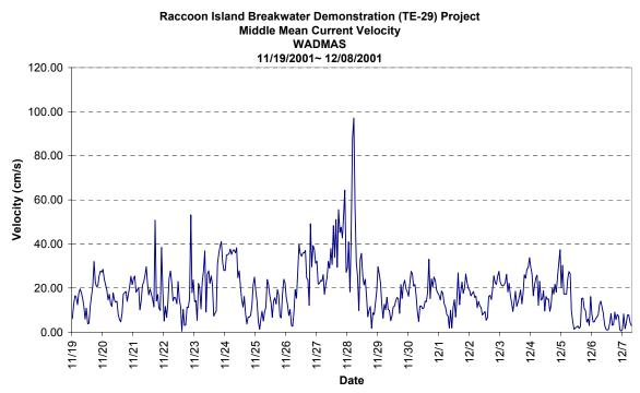
Figure 29. Time series of middle current velocity at D6.
