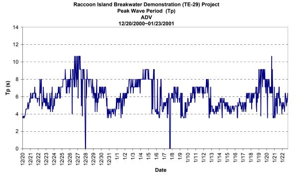
Figure 15. Peak wave period (Tp) at deployment #2 (D2).
