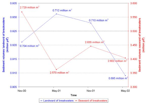
Figure 69. Sediment volume changes of entire areas landward and seaward of the breakwaters.
