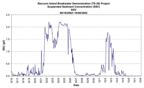
Figure 40. Time series of suspended sediment concentration at D7.
