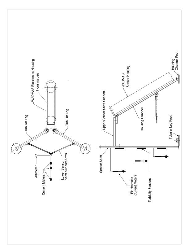
Figure 2. WADMAS sensor platform shown in planform (top) and section (bottom). The array was built by Coastal Studies Institute at LSU and stands  $\sim$  1.5 m (4.92 ft) high.
