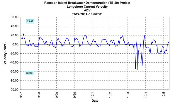
Figure 22. Time series of mean longshore current at D5.
