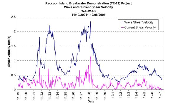
Figure 32. Time series of wave and current bed shear velocities at D6.
