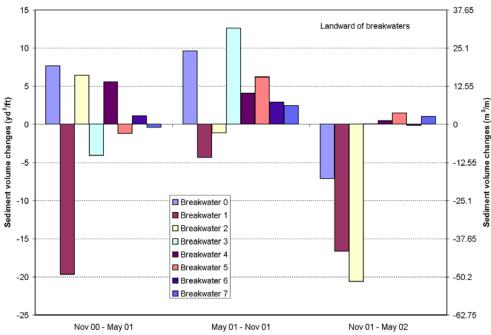
Figure 67. Sediment volume changes of behind breakwater part of the eight survey lines through the breakwaters. Negative values represent erosion, while positive values represent deposition.
