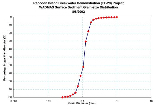
Figure 5. WADMAS surface sediment sample grain size distribution.
