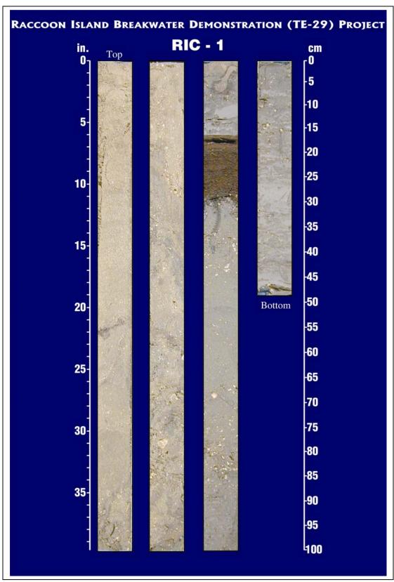
Figure 47. Photograph of core RIC 1 taken from the shoal seaward of the Raccoon Island breakwaters.
