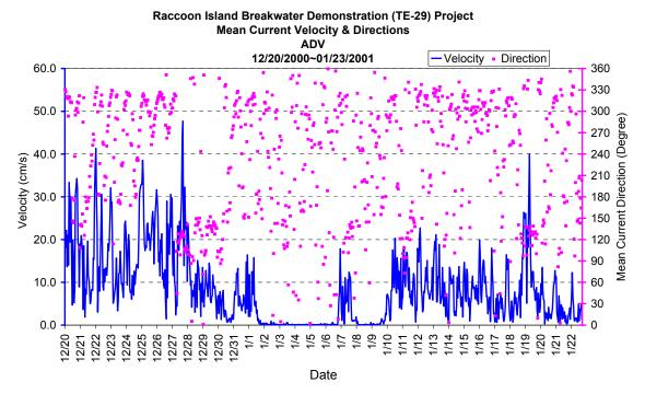
Figure 21. Time series of mean current and directions at D2.
