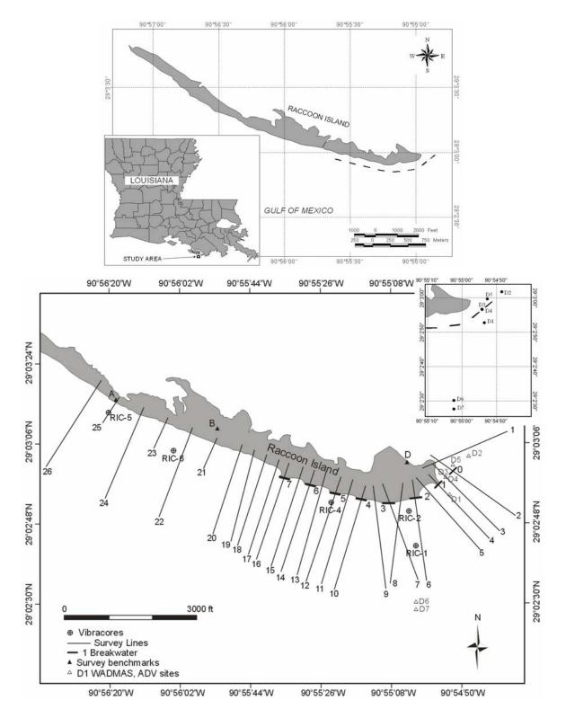
Figure 1. Upper: Study area showing the location of Raccoon Island and the breakwaters along the eastern end of the barrier. Lower: Study area, showing the location of WADMAS, ADV, Sea Gauge, vibracores, and topographic/bathymetric survey lines discussed later in text. Shoreline is based on an aerial photograph taken on 2-6-2002 by the USGS.
