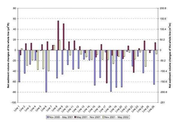
Figure 66. Summaries of sediment volume changes of each survey line during the three survey seasons. Negative values represent erosion, and positive values represent deposition.
