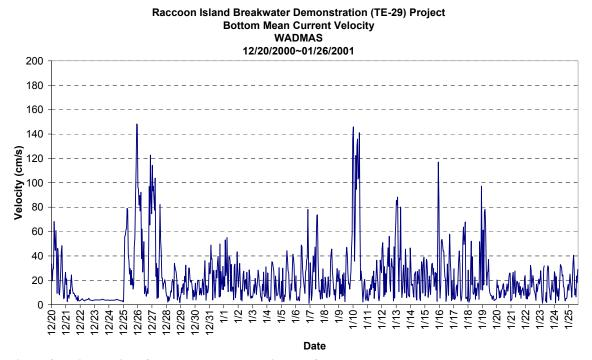
Figure 27. Time series of bottom current velocity at D3
