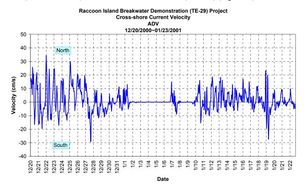
Figure 18. Time series of mean cross-shore current at D2.
