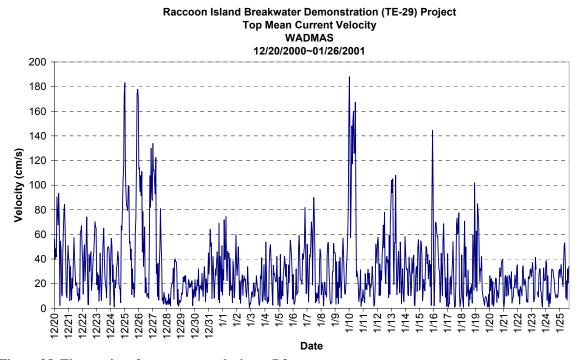
Figure 25. Time series of top current velocity at D3
