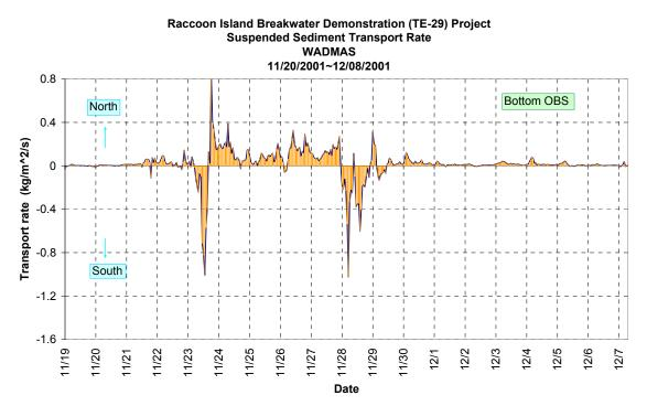
Figure 33. Time series of bottom cross shore suspended sediment transport rate at D6.
