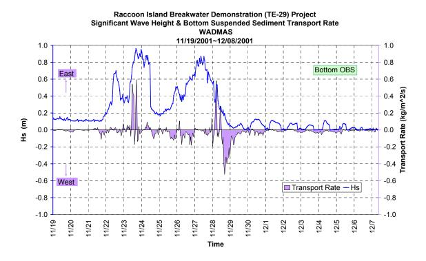
Figure 38. Time series of significant wave height and longshore suspended sediment transport rate at D6.
