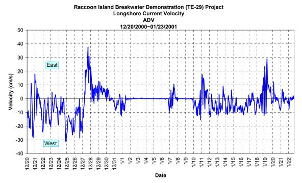
Figure 19. Time series of mean longshore current at D2.
