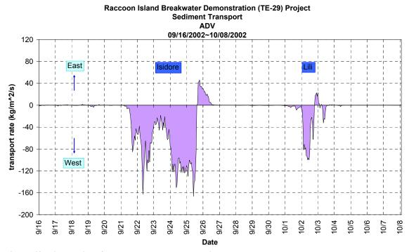
Figure 42. Time series of cross shore suspended sediment transport rate at D7.
