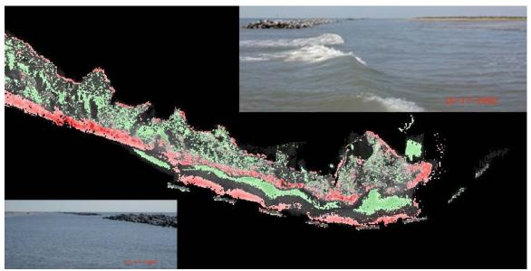
Figure 54. Images of Raccoon Island breakwaters in 2002 after Tropical Storm Isidore and Hurricane Lili. Red color on Lidar image represents erosion and green color represents deposition (Courtesy of Dr. A. Sallenger, USGS).
