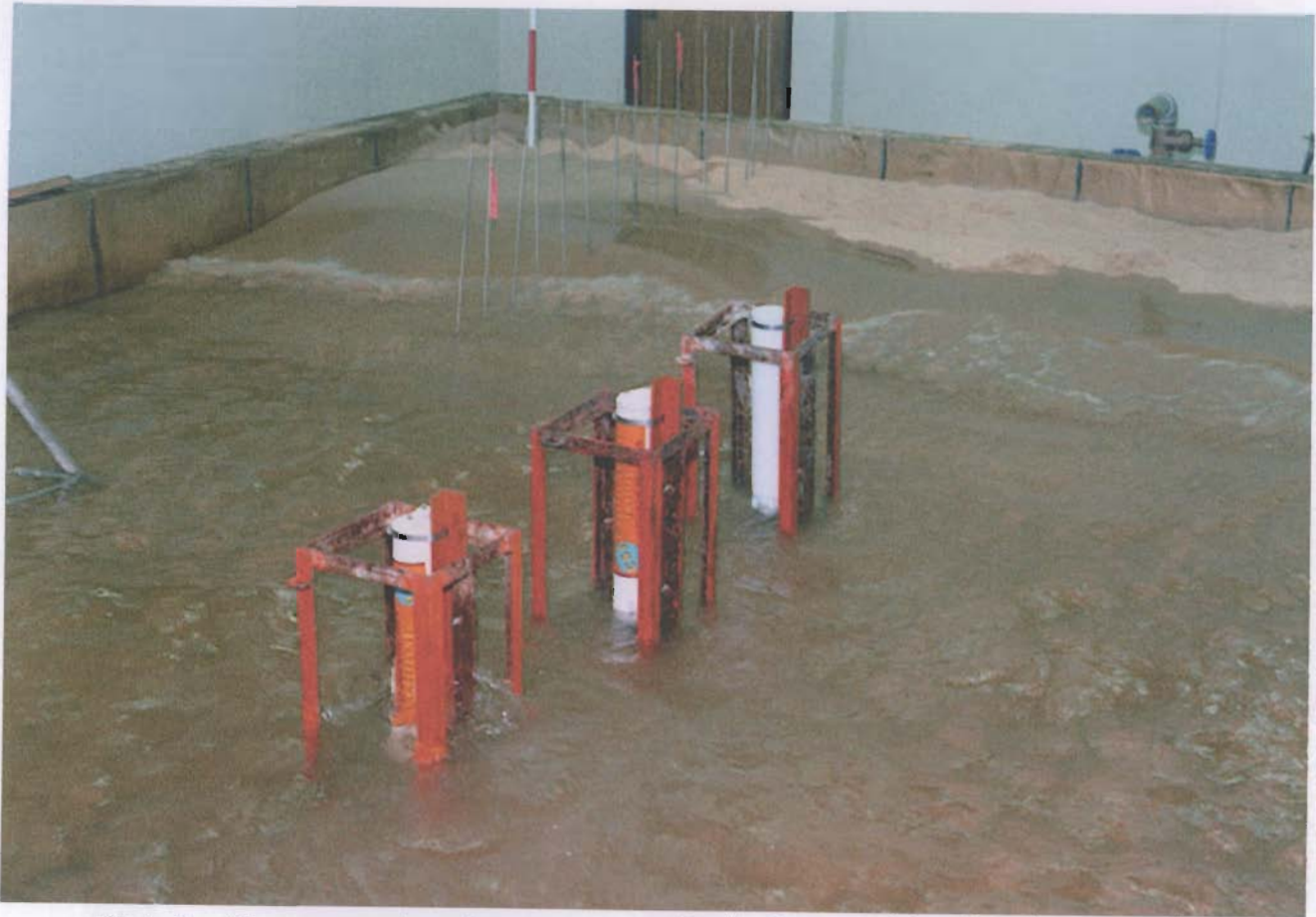
Plate 1. The pressure transducer arrays used in the Raccoon Island breakwater study. The pressure sensors and solid-state recorders are housed in a water-tight casing and are being tested in the Coastal Studies Institute's Wave Simulation Facility.
