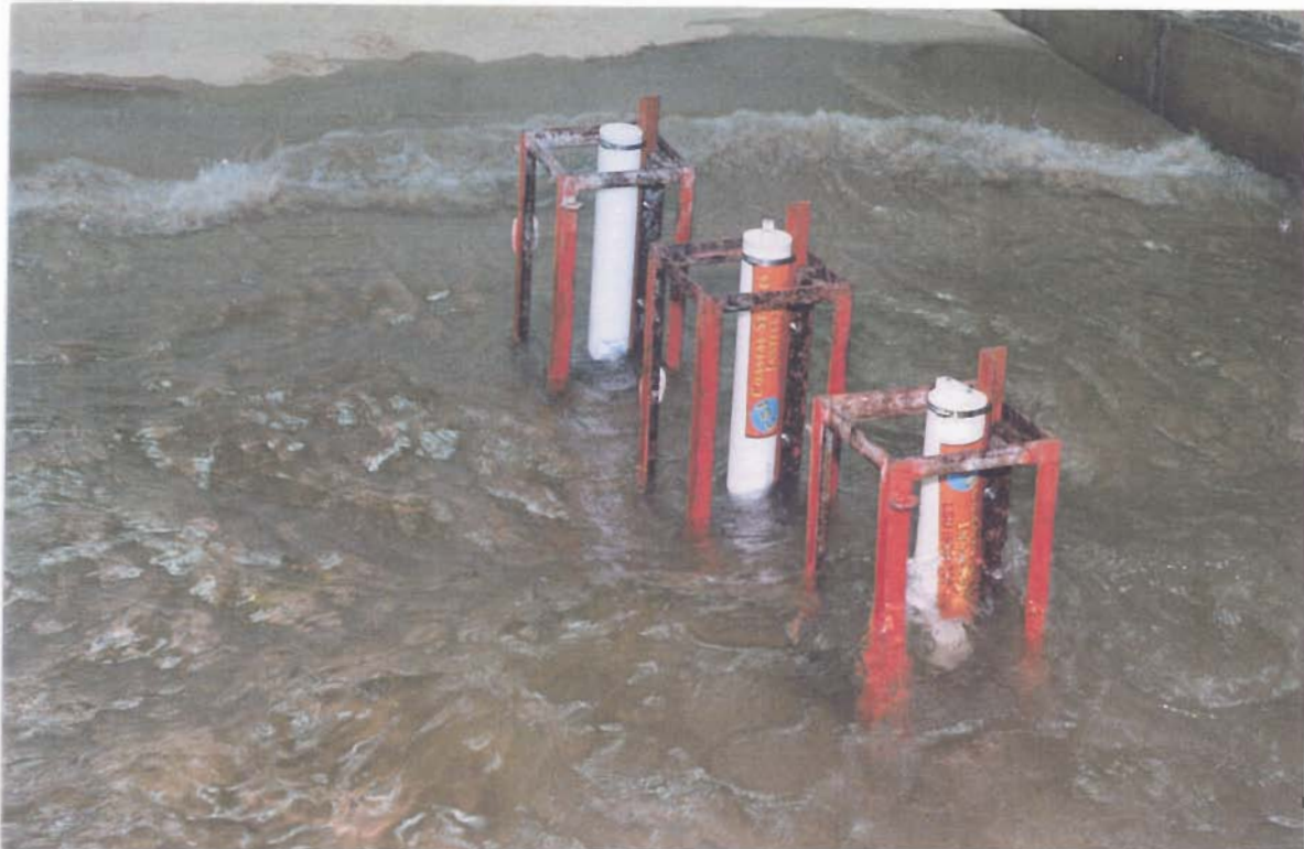
Plate 1. The pressure transducer arrays used in the Raccoon Island breakwaters study. The pressure sensors and solid-state recorders are housed in the water-tight housing and are being tested in the Coastal Studies Institute's Wave Simulating Facility.
