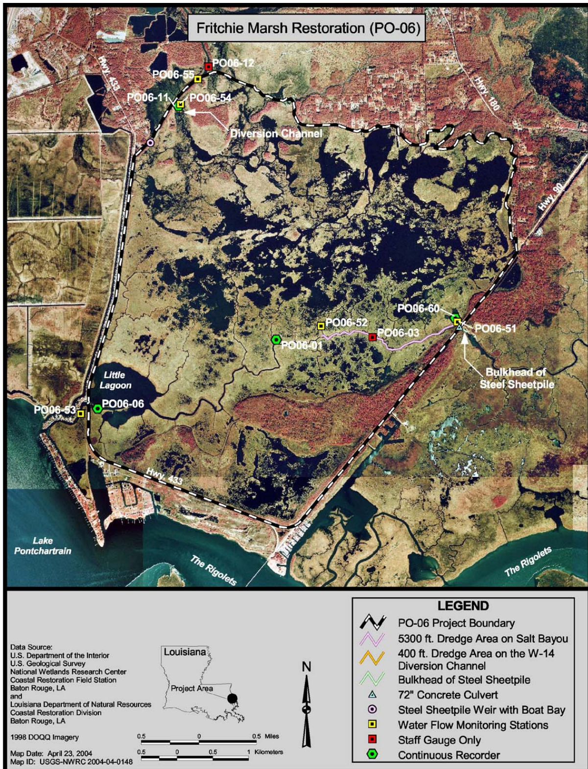
Figure 1. Fritchie Marsh Restoration (PO-06) project boundary, construction features, continuous recorder and staff gauge locations, and water flow monitoring locations.
