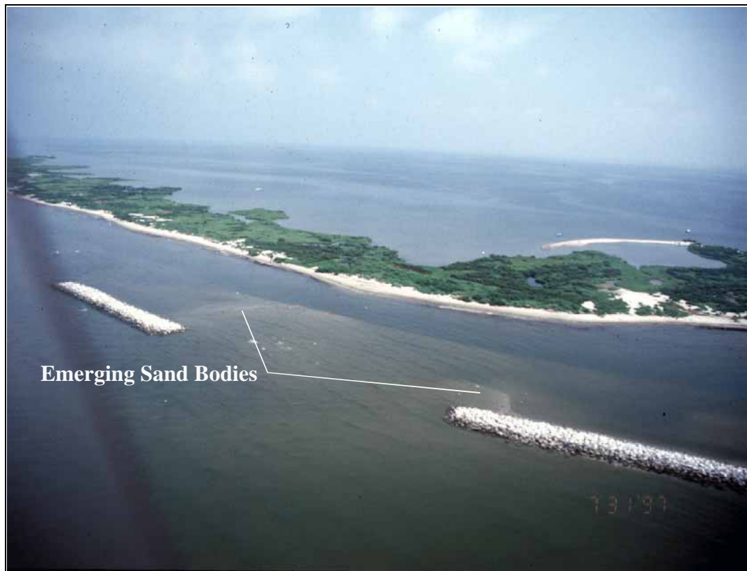
Figure 16. Sediment accumulation in the lee of breakwaters 3 and 4 less than two weeks after construction was completed (photograph taken 31 July 1998).
