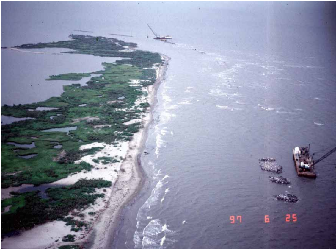
Figure 10. Rapid salient development in the lee of breakwater 7 during construction of the detached, segmented breakwater system at Raccoon Island, Louisiana.
