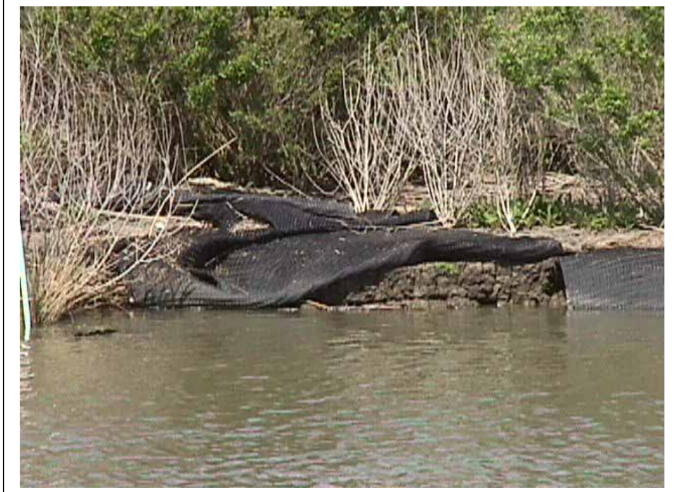
Figure 8. Geo-mesh fabric laid on shore (design F; treatment 3) at Falgout Canal - Vegetative Plantings Demonstration Project (TE-17). Fabric has been tossed up on shore due to wave action. (Photo taken March 13, 2000).
