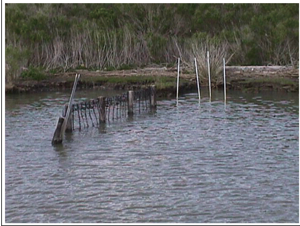
Figure 15. Damage on Shore-perpendicular, four section uniaxial geo-grid fence (design D; treatment 4) at Falgout Canal - Vegetative Plantings Demonstration Project (TE-17) (Photo taken March 13, 2000).
