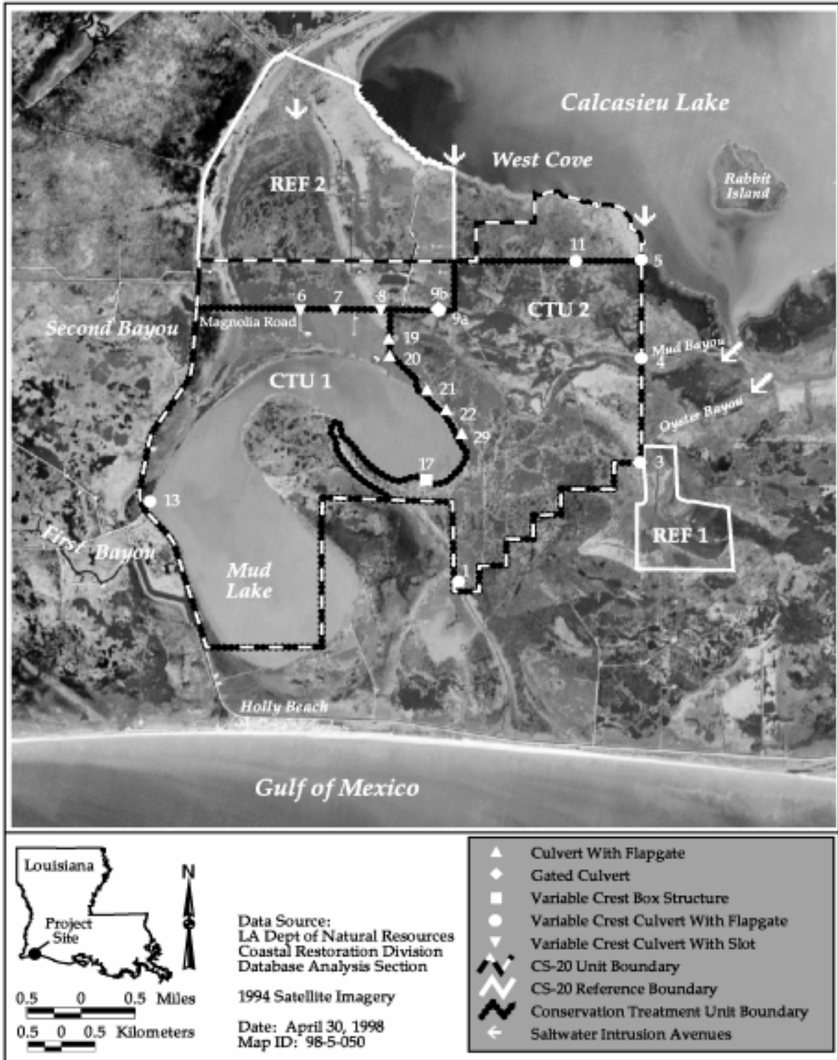
Figure 1. East Mud Lake (CS-20) project map depicting project boundaries, conservation treatment unit boundaries, reference area boundaries and project features.
