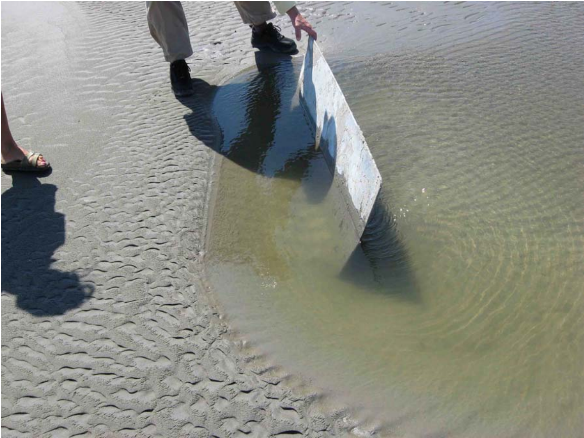
Photo #4 – Settlement Plate (overturned).
