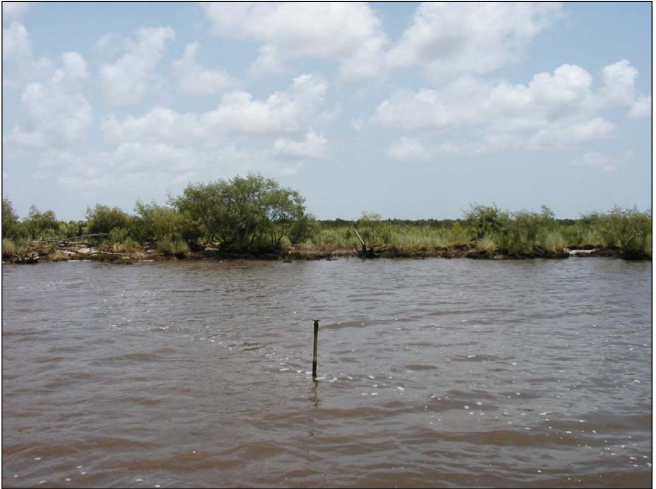
Figure 15. View of the Freshwater Bayou Canal shoreline at reference area R2 (north unit) monitoring station ME13-25R taken on July 21, 2003. Note the current shoreline position which is 89.0 ft (27.1 m) inland from the survey hub in open water in the foreground. The hub was placed 44.7 feet (13.6 m) inland from the shoreline when it was installed in 1998.
