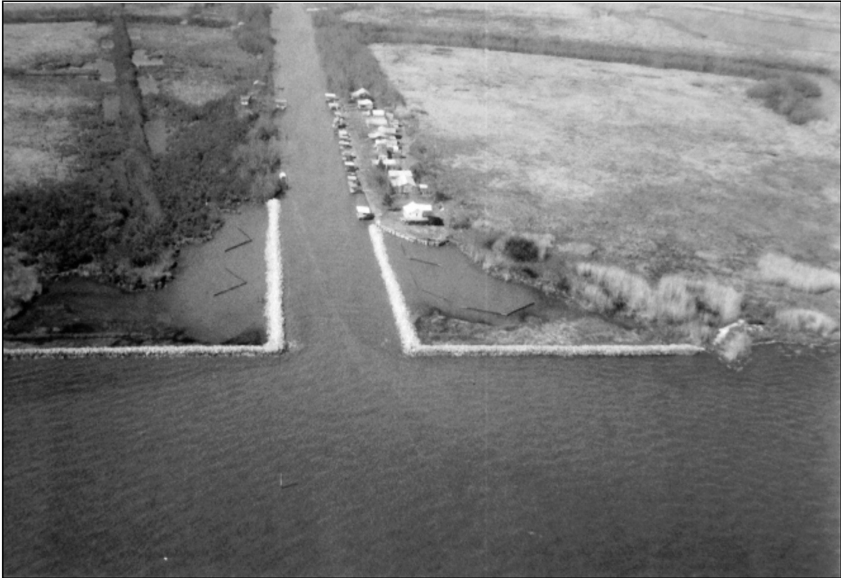
Figure 2. Boston Canal/Vermilion Bay Shoreline Protection (T/V-09) rock breakwaters and sediment fences at the mouth of Boston Canal.
