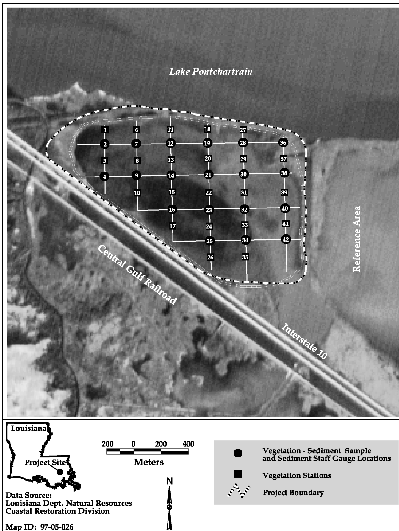
Figure 2. Bayou La Branche Wetland Restoration (PO-17) project vegetation stations, sediment stations, sediment staff gauges, and elevation survey transects.
