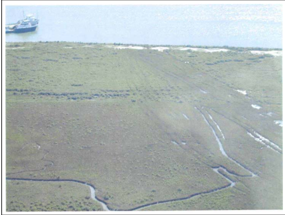
Figure 11. February 2003 aerial view of severe marsh tracks located along Belle Pass in the vicinity of closure 4 at the West Belle Pass Restoration (TE-23) project.
