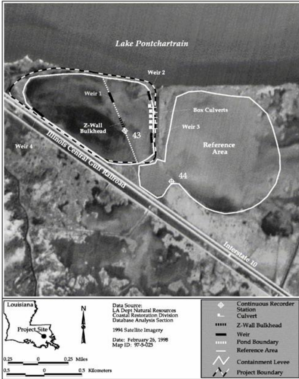
Figure 2. Locations of the Bayou La Branche wetland creation (PO-17) project area, reference area, project features and continuous recorder stations (PO17-43) and (PO17-44R),
