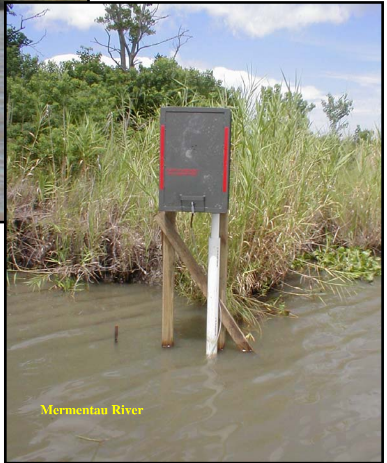
Figure 21: Discharge And Water Level Gauge Installed In The Mermentau River Near Grand Lake.
