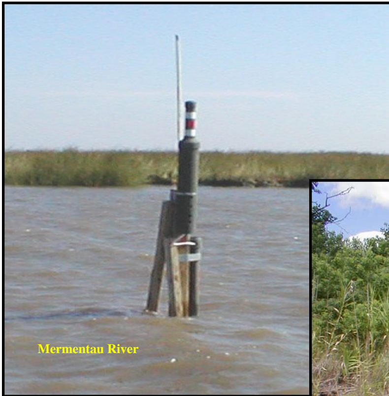
Figure 20: Water Level And Salinity Data Sonde Installed In The Mouth Of The Mermentau River
