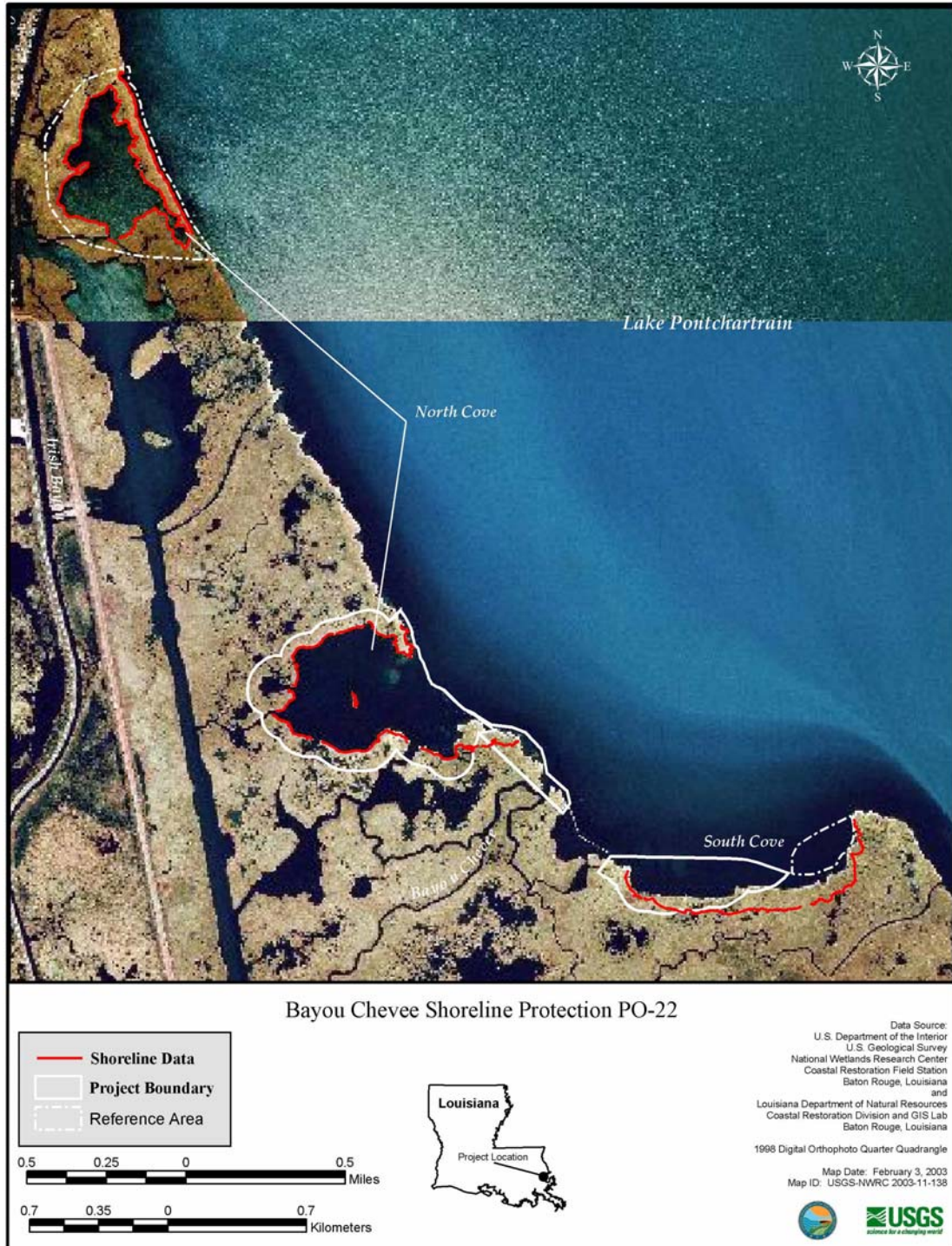
Figure 3. 2001 Shoreline position overlaid on 1998 DOQQ image of the Bayou Chevee Shoreline Protection (PO-22) project.
