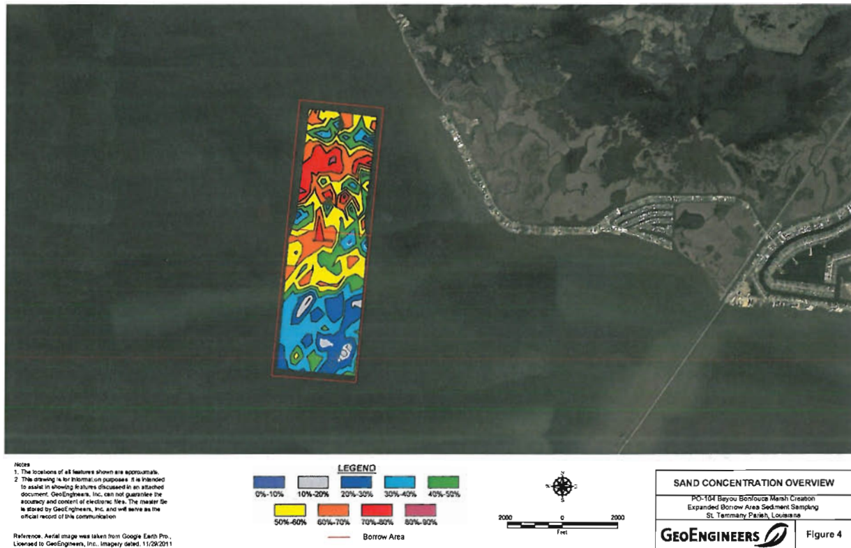
Figure 4. Graphical representation of the distribution of surface sand content within the proposed borrow areas.
