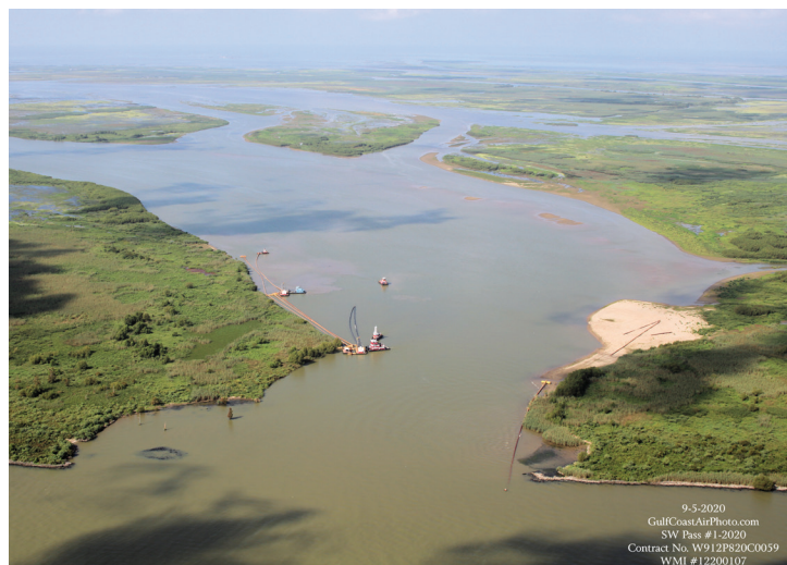
Figure 16. A view towards the southwest at the entrance of the West Bay Sediment Diversion (MR-03). A mature network of distributary channels weaves through naturally formed and engineered features in West Bay that are no longer distinguishable. Equipment staged at the diversion's entrance prepares to distribute dredged material to various parts of the system.
