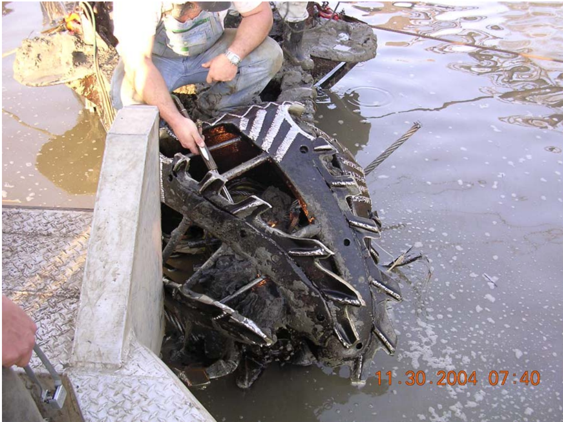
Photo 17. Cutting cable from cutterhead.
