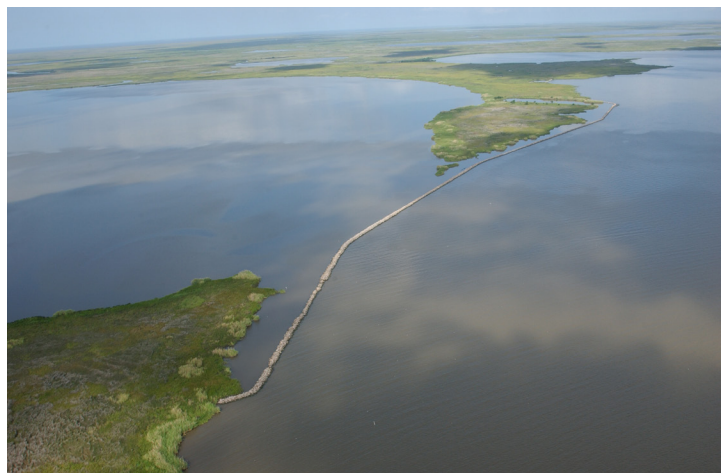
Project features include shoreline protection, canal closures, and isolation of Lake Sand from Vermilion Bay with a rock dike on the northeastern edge of Marsh Island. View is looking west.
