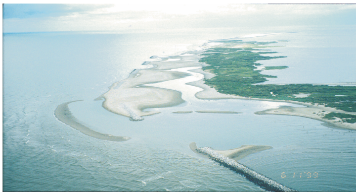
Sand deposits or "tombolos" have developed behind the breakwaters that protect and enhance the island. A less dramatic, however still positive effect, is expected to occur behind the 8 additional breakwaters being constructed to the west of the existing breakwaters.
