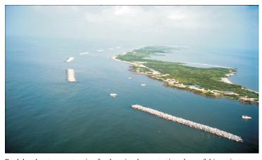
Rock breakwater construction for the prior demonstration phase of this project was completed on the east end of the island in June 1997. Taken immediately after construction was complete, this 1997 photograph shows no sand behind the breakwaters.
