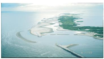
Sand deposits or "tombolos" have developed behind the breakwaters that protect and enhance the island. A less dramatic, however still positive effect, is expected to occur behind the 8 additional breakwaters being constructed to the west of the existing breakwaters.
