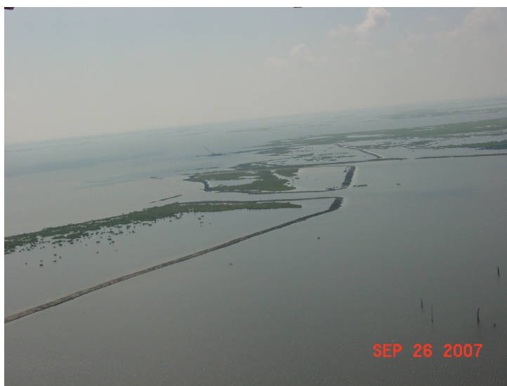
Aerial view of the interior (back) containment dikes that have been constructed to contain dredged material for the purpose of marsh creation. In order from front to back are the northern, central, and southern sections.
