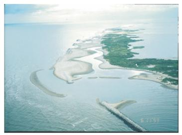
Segmented rock breakwaters function as effective barriers against perpetual wave erosion and act as sand traps. Newly formed "tombolos," or sandbars, can be seen behind the breakwaters.
