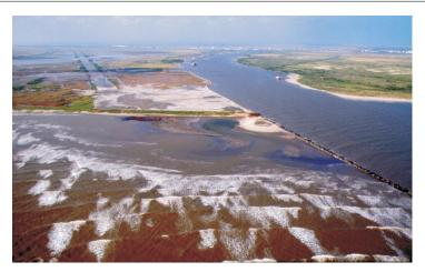
In the photo above, the Gulf of Mexico is in the foreground, and Belle Pass is the wide channel that can be seen curving off to the right near the top of the image. The riprap dike that was constructed runs along its western bank. The brown, white, and green areas just above the gulf's shoreline and to the left of Belle Pass is where the deposited dredge material has promoted newly emergent marsh.
