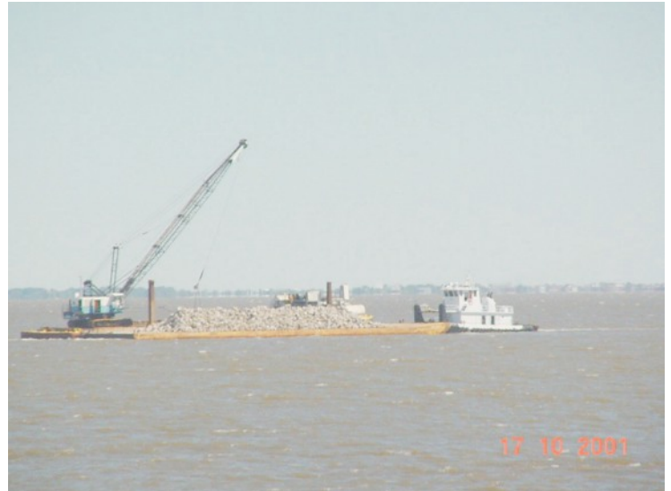
Fully-loaded barge of rock waiting to be unloaded at Bayou Chevee construction site.
