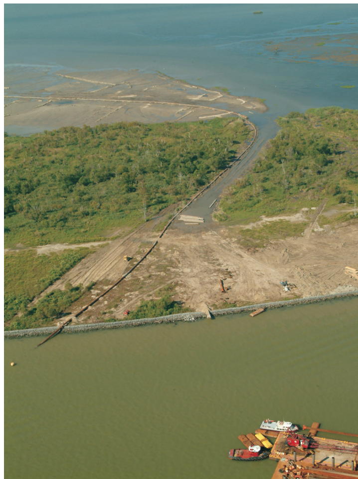
A dredge is being used to create marsh in the lower delta for the West Bay Sediment Diversion (MR-03) project. Work similar to this will take place during construction of the Benneys Bay project.
