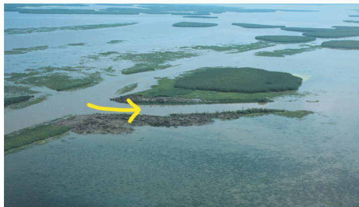
The arrow shows how water and sediments flow through a crevasse in the Mississippi River.
