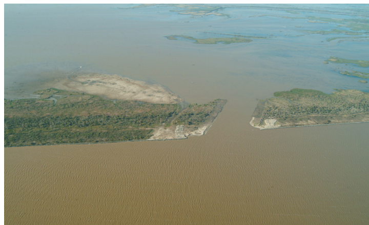
The conveyance channel allows fresh water and sediment to flow from the Mississippi River (bottom of picture) to restore vegetated wetlands in an area that is currently shallow open water.
