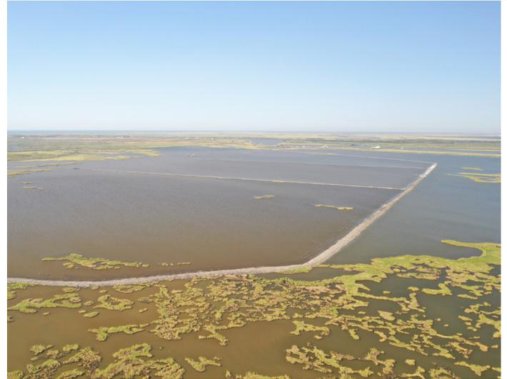
Photograph of the external and internal containment dike construction progress of the No Name Bayou Marsh Creation and Nourishment project.
