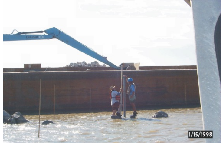
Settlement plates such as the one pictured here will be used to determine if settling of the structure has occurred. Technicians from NRCS's Crowley Watershed Office are shown taking baseline elevations before more rock is deposited. Future elevation readings will be taken after the structure is completed.
