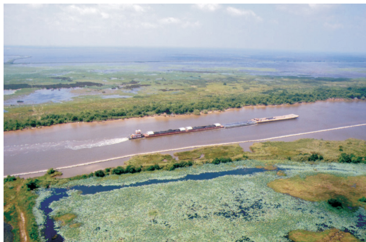
Rock riprap provides shoreline protection from wave energy produced by shipping vessels on the GIWW.
