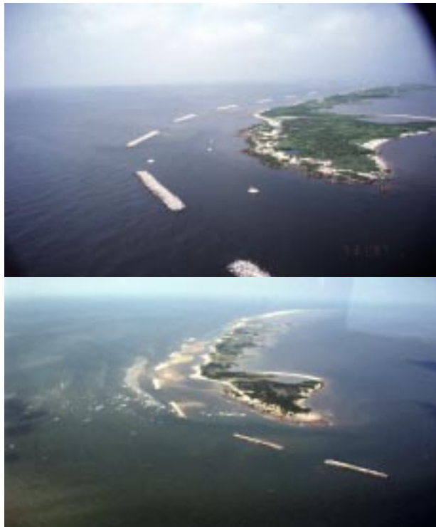
Raccoon Island (TE-29) immediately after construction of segmented breakwaters in 1997 (top) and one year after construction in 1998 (bottom).
