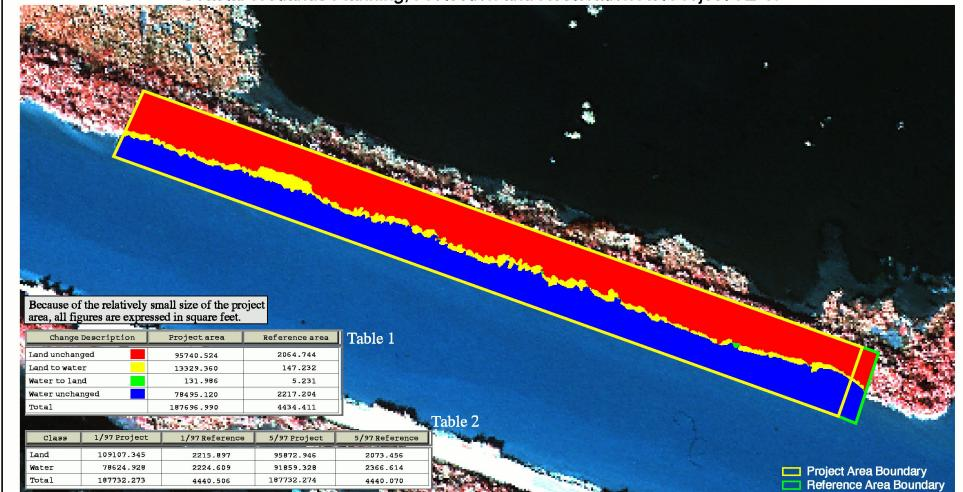
Land/water analysis derived from 1:12,000 scale color-infrared aerial photography taken November 8, 1997 and shown here at 1:3,400 scale.
