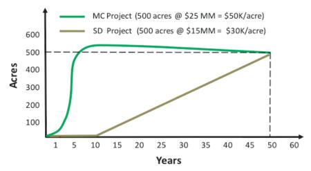
Consider the sample restoration trajectories for marsh creation (MC) and sediment diversion (SD) in the graphic above. Each of these projects converges on a common level of 500 net acres of coastal land in 50 years. If we consider final costs and acreages only, the SD project is the apparent better deal, with a cost of \$30K/acre compared to \$50K/acre for the MC project.
