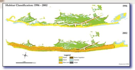
**Figure 1:** Habitat classification maps showing Trinity Island before and after the restoration project was completed. The "bare land" area on the bottom section of the map is the sediment that was pumped onto the island. done by CWPPRA, the Coastal Wetlands Planing, Protection and Restoration Act.
