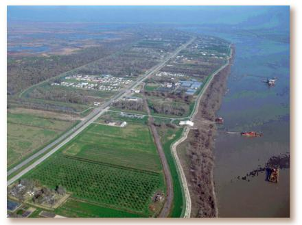
Sediment is used from the Mississippi River to rebuild wetlands in a new location. The red boat near the levee is pumping sediment to the fragile wetlands in top left of the image. The sediment is then used to rebuild marsh that had turned to open water, creating new wetlands.
