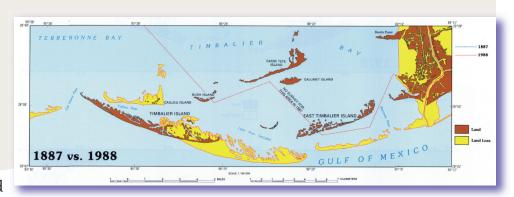
to just as Timbalier Island). Erosion due to subsidence, lack of sediment, sea level rise, waves, and winds from many storms has reduced the land area of the islands dramatically, while the natural migration has moved the islands towards the mainland. In addition, oil and gas exploration and production has been particularly active at East Timbalier Island. Canals and disturbance of the land for drilling have added to the loss that is taking place in this area.
