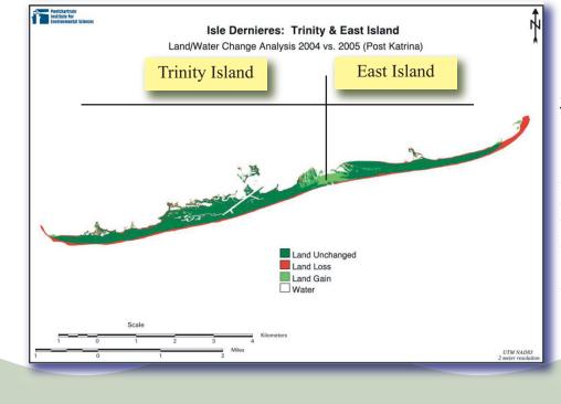
**Figure 2:** Land loss map showing Trinity and East Islands, now joined together by sediment deposition after hurricanes Katrina and Rita. The red area is the sediment lost due to the storm surges. The lighter green areas represent sediment deposition due to the storms.
