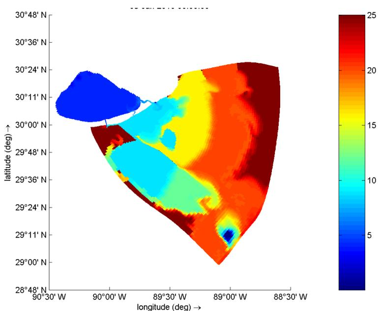
Figure 7.1 Initial salinity (parts per thousand) in model based on measurements
