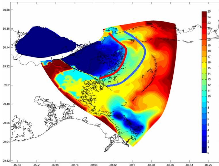
Figure 7.11 The 10 ppt and 15 ppt isohaline for the diversion scenario
