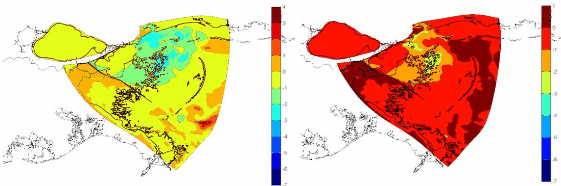
Figure 7.10 Difference plot of salinity between 3-year simulation with Violet Diversion and without diversion flow in the upper layer (left) and bottom layer (right), both with MRGO closure structure. Positive values indicate an increase in salinity.
