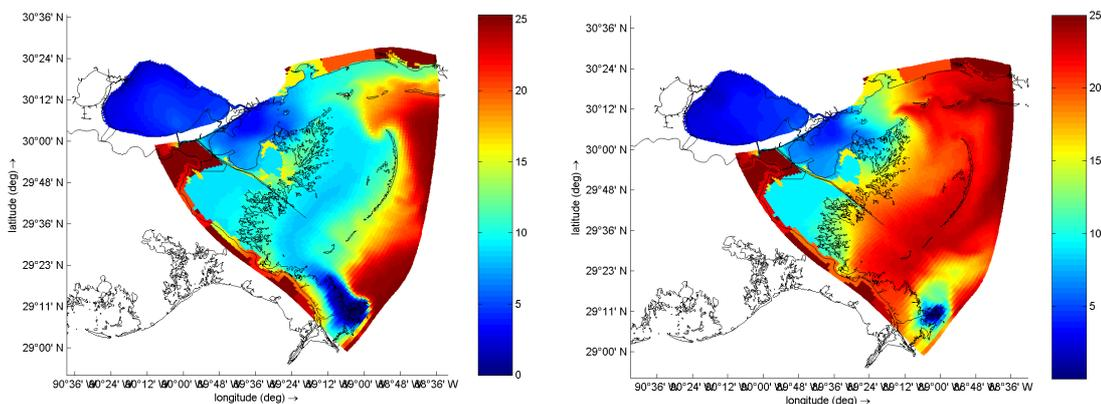
Figure 7.2 Salinities after 2 months simulation in depth averaged model (left) and in top layer of 3D modeling with 10  $\sigma$ -layers (right)
