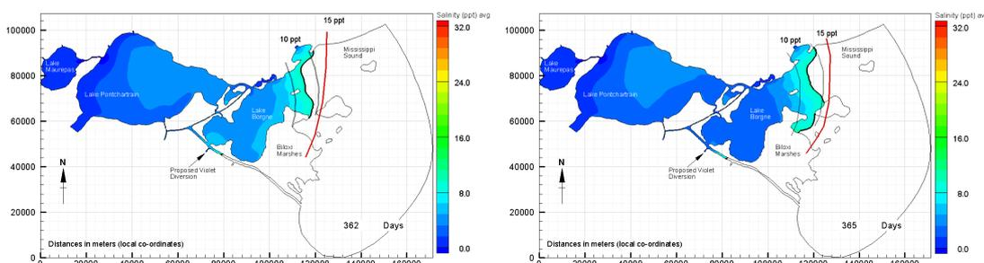
Figure 6.20 Surface salinities in Lakes Borgne and Lake Pontchartrain after a simulation of a year for the annual 5,000 cfs scenario (left) and annual 15,000 cfs scenario (right) (Georgiou et al., 2007)
