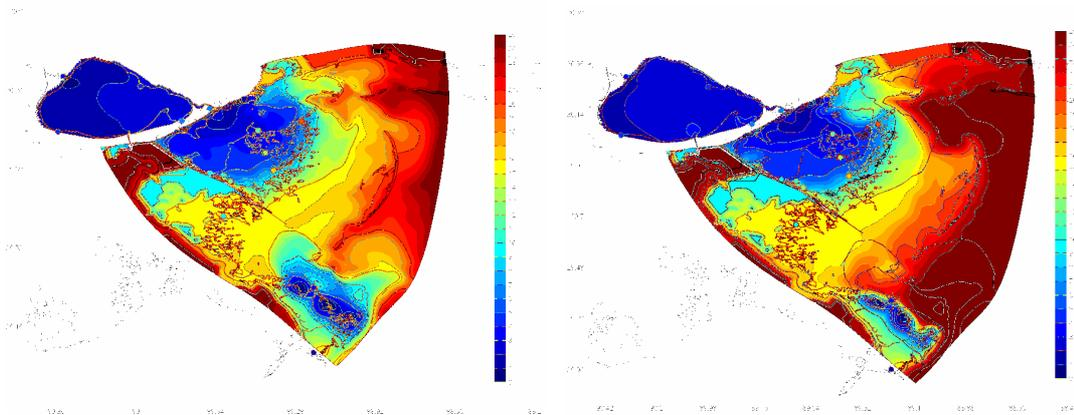
Figure 7.5 Salinity in upper layer (left) and bottom layer (right) after 2 years simulation with baseline conditions. White contour lines are 5 ppt contour lines of upper layer, colored dots are measured yearly averages.
