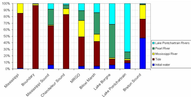
Figure 7.7 Contribution of each source per observation section after 3 years of simulation
