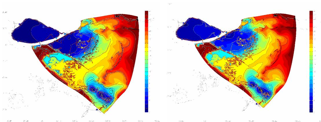
Figure 7.9 Salinity in upper layer after 2 years of simulation with MRGO closure (left) and without MRGO closure (right)
