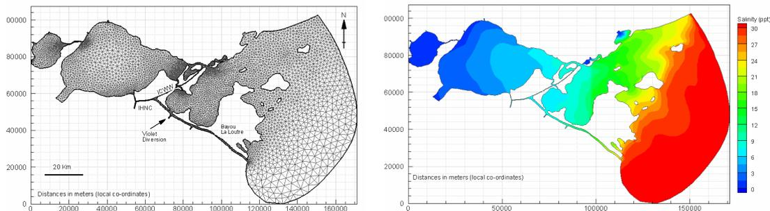
Figure 4.23 Model domain (left) and initial salinity (right) of the FVCOM model (Georgiou et al., 2007)
