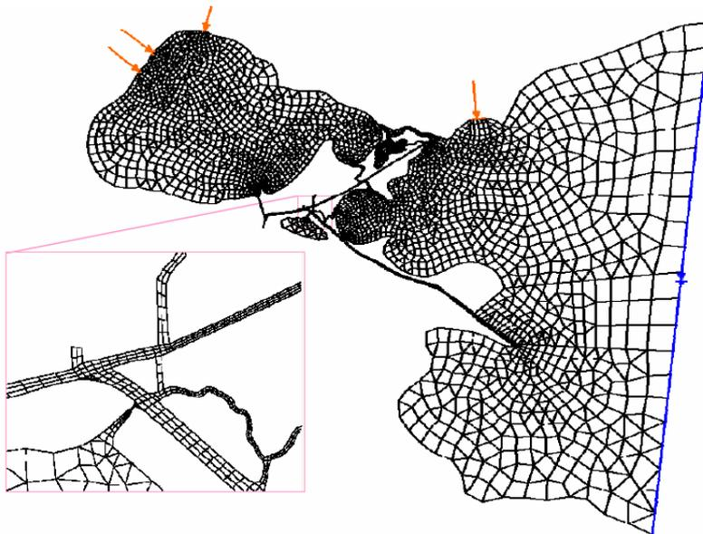
Figure 4.24 Model domain with computational mesh for modeling of flow velocities near the IHNC storm surge barrier. Zoom-in is the location of the barrier (AECOM, 2009)
