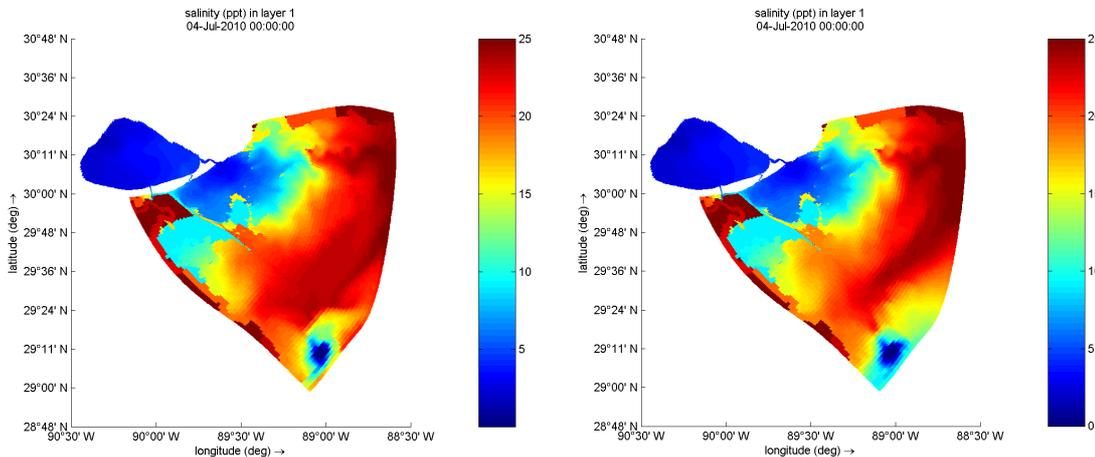
Figure 7.4 Salinity after 6 months simulation with uniform (25 ppt) boundary (left) and spatially varying boundary (right)
