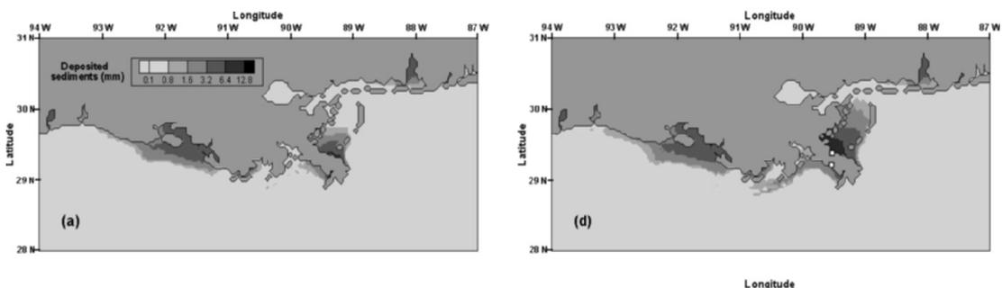
Figure 6.16 Deposited sediment thickness converted to yearly rates under existing conditions (left) and a 70-30 (west – east) diversion ratio (right) (Rego et al., 2010)
