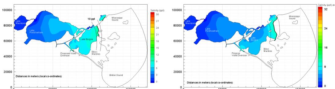
Figure 6.19 Surface salinities in Lake Borgne and Lake Pontchartrain after a simulation of a year with open MRGO (left) and with completed MRGO closure structure (right) (Georgiou et al., 2007)
