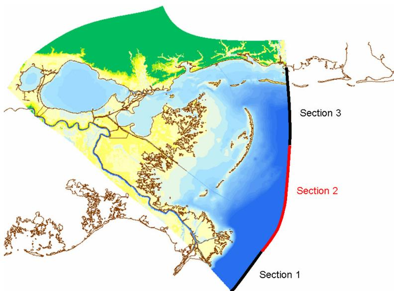
Figure 7.3 Section for differentiation of salinity over model boundary
