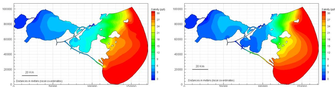
Figure 6.18 Salinities in Pontchartrain Basin calculated with FVCOM in baseline condition (left) and with 10,000 cfs diversion scenario at Violet (right) (Georgiou et al., 2007)
