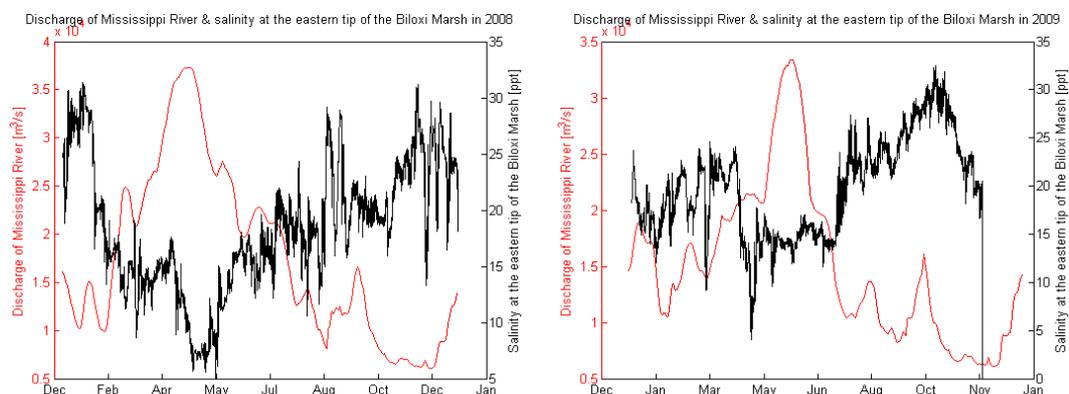
Figure 6.14 Discharge of Mississippi River versus salinity in the eastern tip of the Biloxi Marshes in 2008 (left) and 2009 (right)
