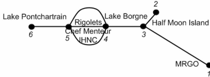
Figure A.1 Schematization of the Pontchartrain Basin for application of harmonic method
