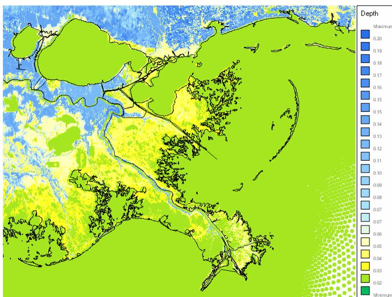
Figure 5.3 ADCIRC SL15 roughness values (Manning coefficient)
