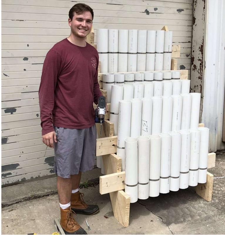
Figure 5. Marsh organ design with 5 elevation treatments and 8 mesocosms per row used during the 2021 growing season. Similar designs were used for all the other growing season experiments
