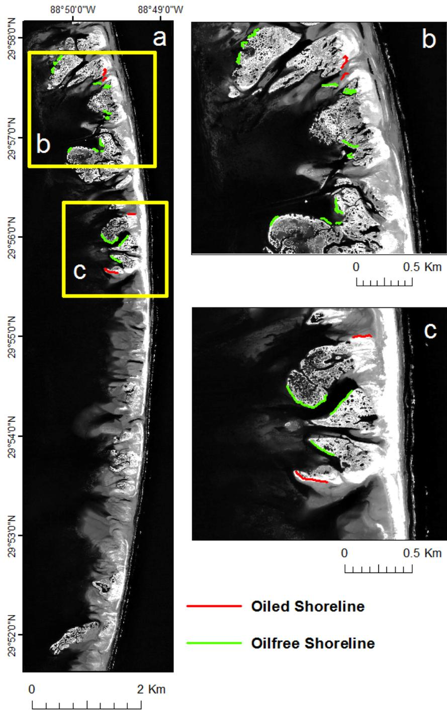
**Figure 3.** (a) SCAT oiled and oil-free shoreline data selected for analysis overlaid on the AVIRIS flightlines acquired over Chandeleur Islands on September 21, 2010 with detailed views of two sections, (b) and (c) affected by oiling.
