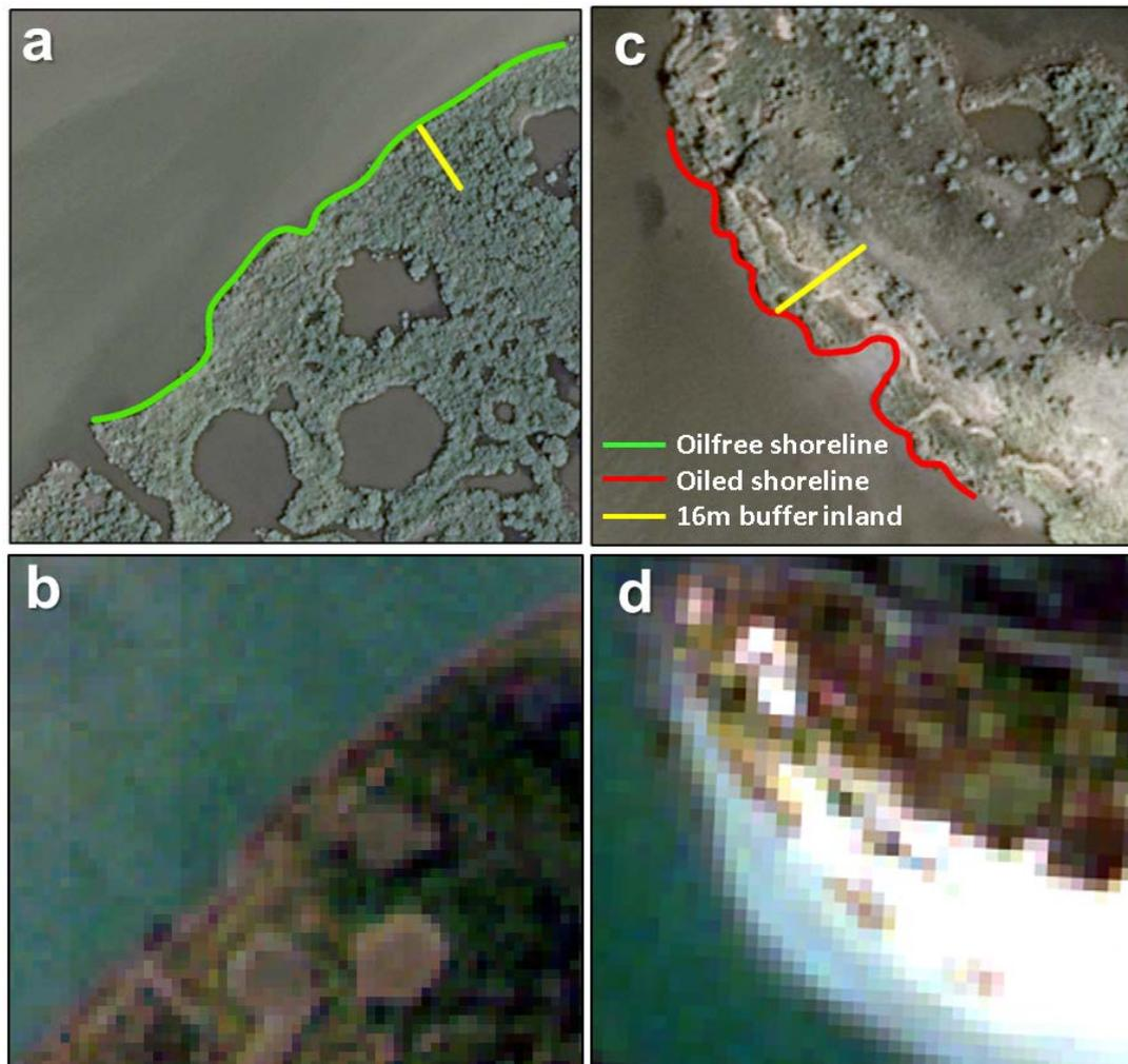
**Figure 6.** (a) SCAT shoreline data overlaid on 2010 GIS Aerometric 0.3 m imagery of a section of Chaudet Islands with a yellow line marking the extent of the 16 meter buffer used in the analyses, (b) AVIRIS true color image showing the same extent of (a) at 7.7 m resolution, (c) SCAT shoreline data overlaid on 0.3m imagery of a section of Chaudet Islands, (d) AVIRIS true color image showing the extent of (c) at 7.7 m resolution.
