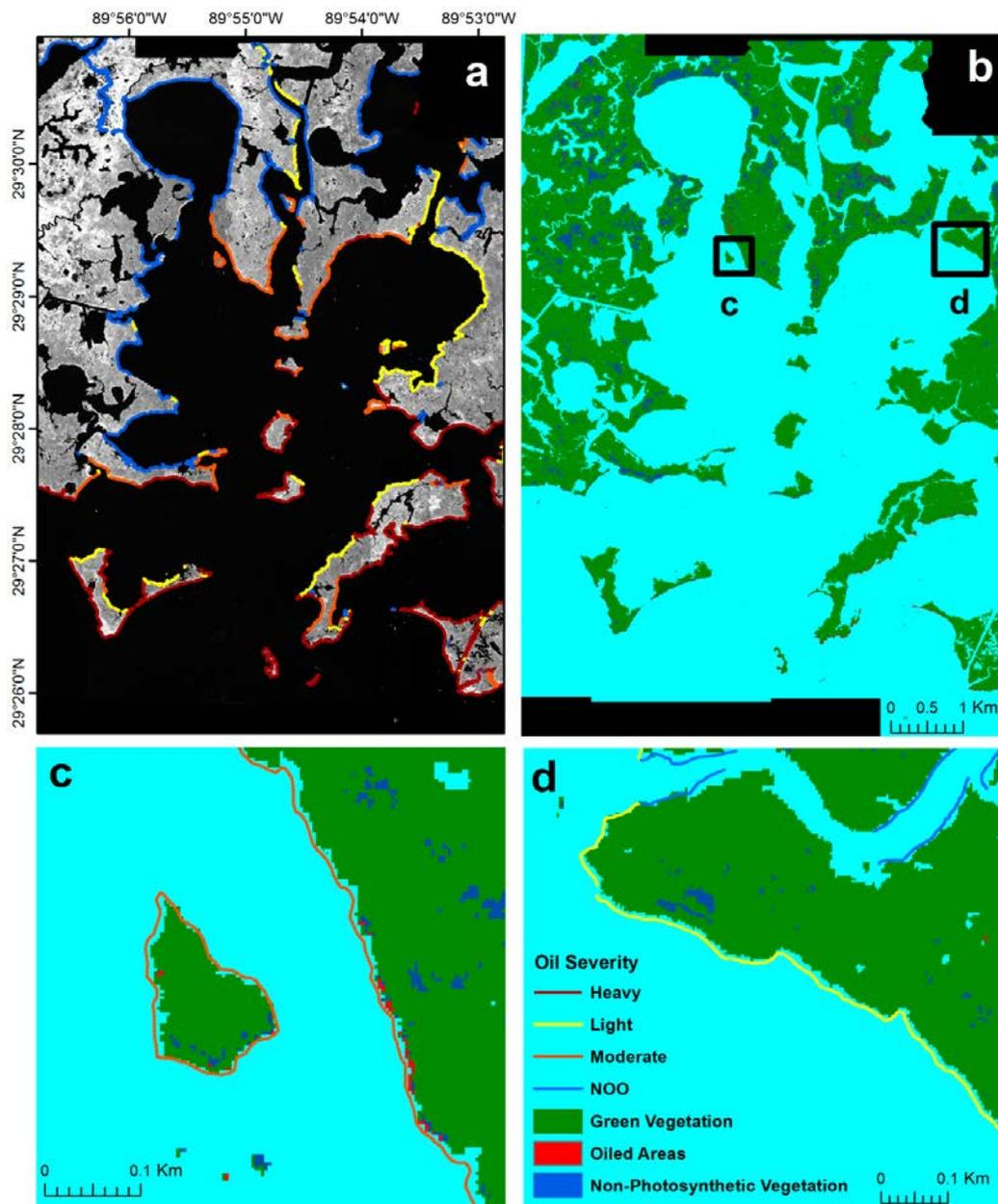
**Figure 2.** (a) SCAT oiled shoreline data overlaid on the AVIRIS flightlines acquired September 14, 2010 over Barataria Bay, (b) landcover classification showing location of inset c and d, (c) a shoreline designated as moderately oiled by SCAT, with patches of oiled pixels, and (d) a shoreline designated as lightly oiled by SCAT with very few oiled pixels.
