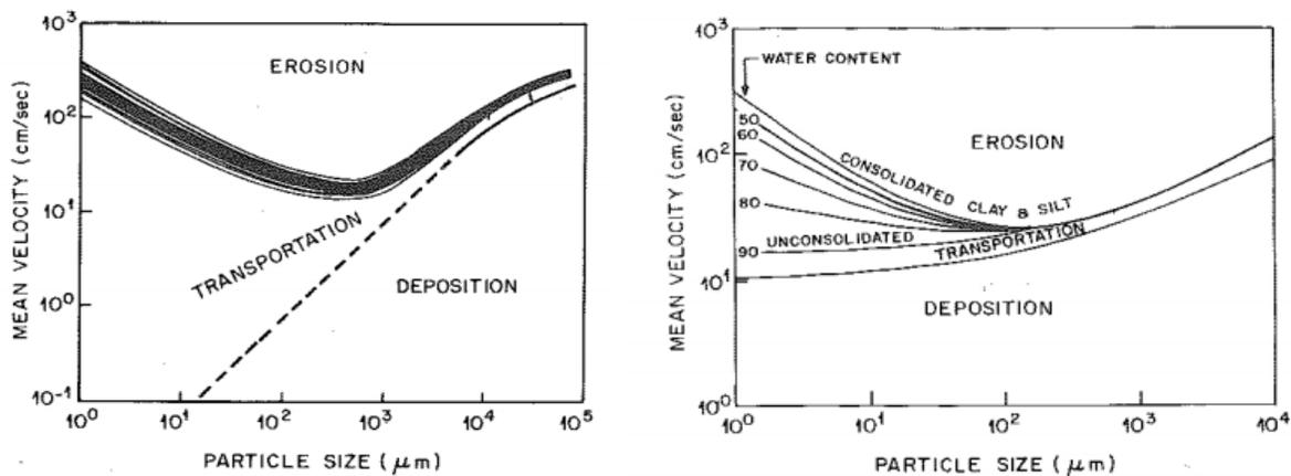
Figure 4.3. Hjustrom (left) and Postma (right) diagrams, modified from Dade et al., (1992). Both plots illustrate the mean velocity necessary to transport particles of a specific size. Note the increase in velocity needed to erode consolidated cohesive sediment.
