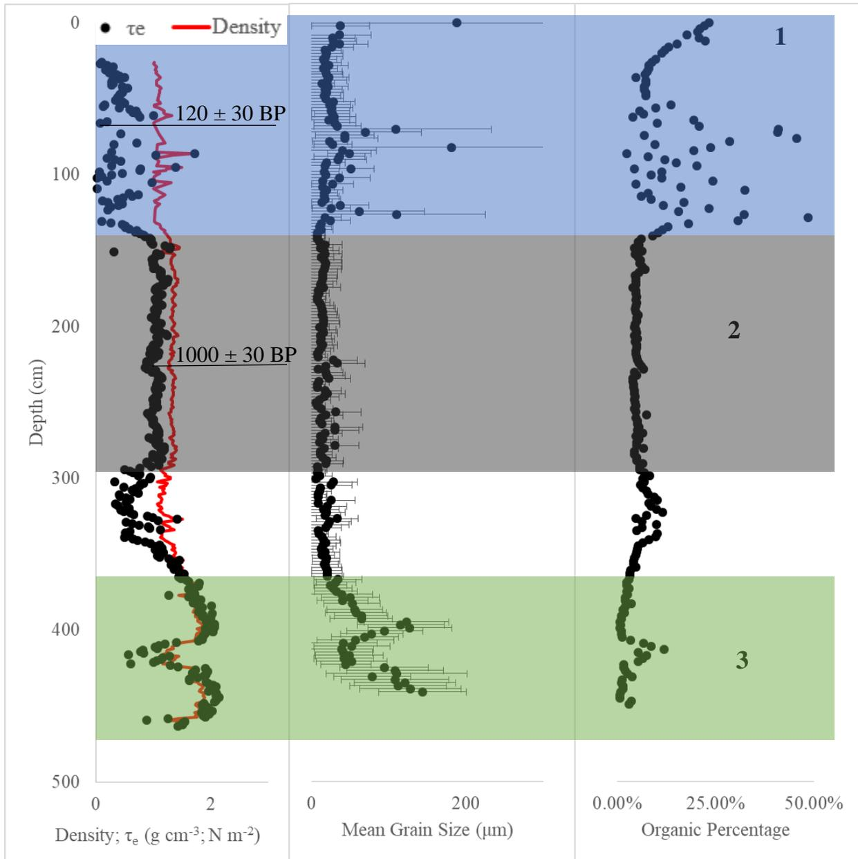
Figure 4.6. Bulk density from the gamma logger, critical erosional shear stress ( $\tau_e$ ), mean grain size, carbon dates, and dry mass organic in core TER 1T. Three prominent facies are visible in most vibracores. Facies 1 is unconsolidated/fluid sand and mud with low erosional resistance; 2 is consolidated mud with moderate to strong erosional resistance; 3 is sandy deposits with high erosional resistance. Note chaotic pattern midway through Facies 1.
