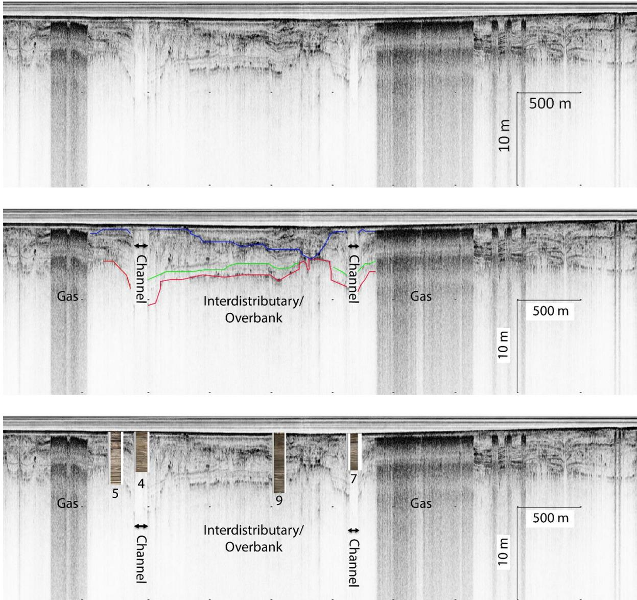
Figure 4.5. Top is an uninterpreted seismic profile of transect A – A'. Middle is the author's interpretation of the profile. Bottom contains the four most proximal vibracores (labeled 4, 5, 7, 9).
