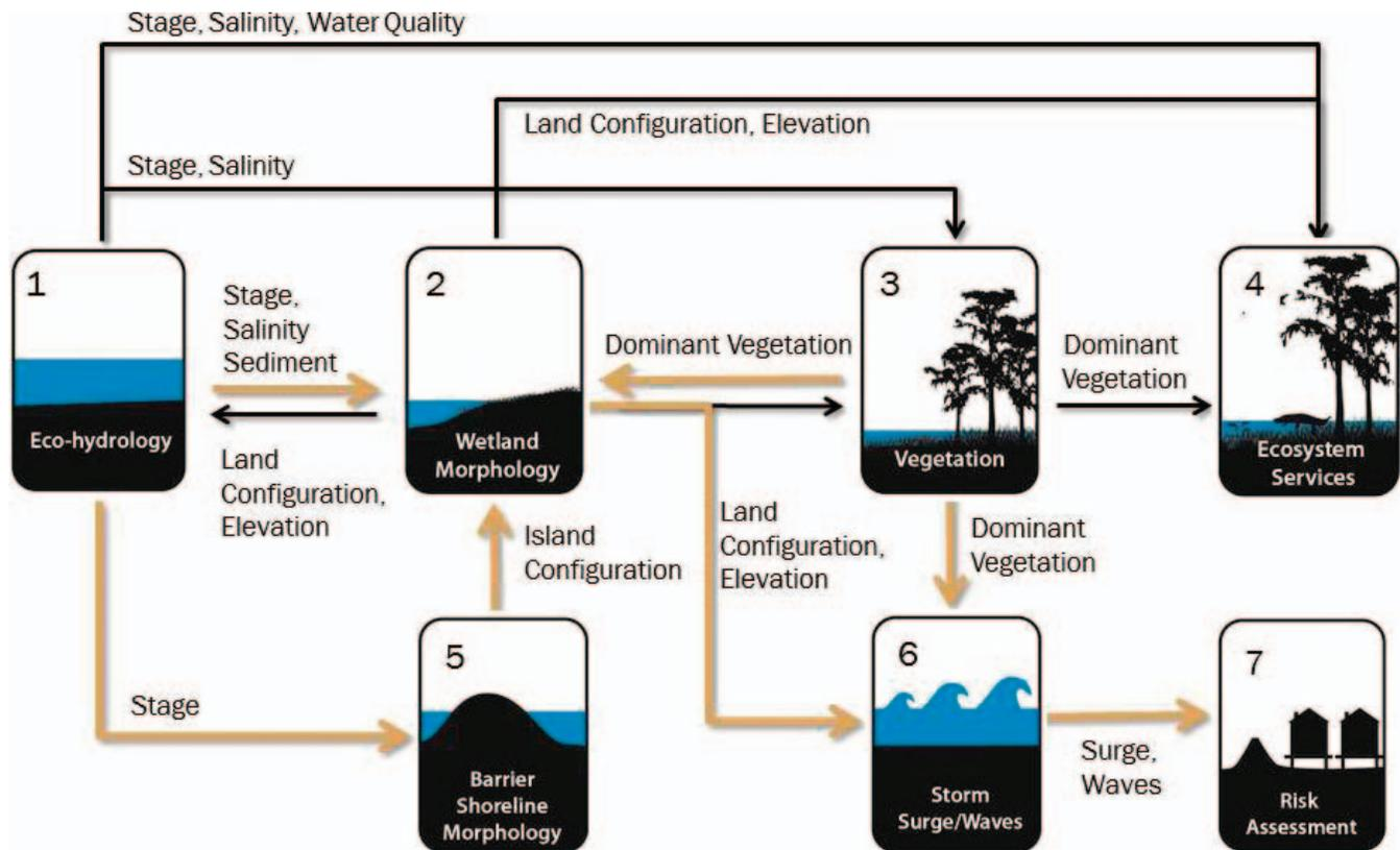
Figure 3. The modeling framework for the 2012 Coastal Master Plan used a series of integrated, coastwide predictive models within a systems context (CPRA, 2012, Appendix D). The main input and outputs of each model that are linked to other models are indicated. The yellow arrows indicate substantially improved or entirely new feedback and links developed and utilized to support the 2012 Coastal Master Plan process.
