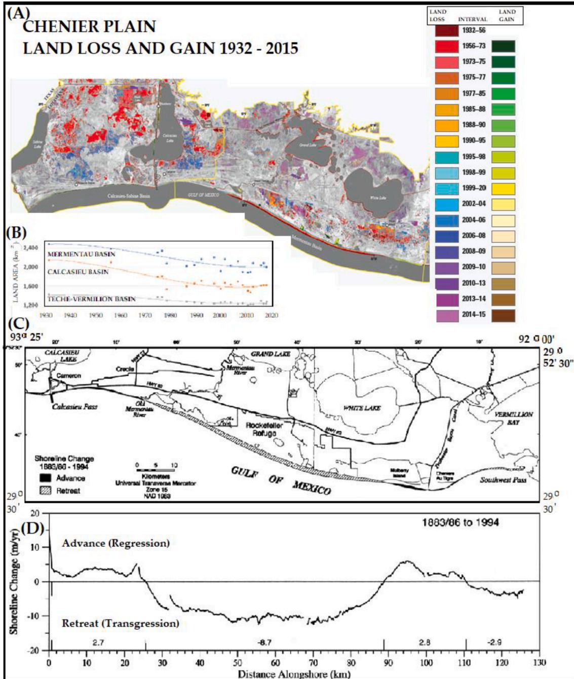
Fig. 6. (A) Map showing land loss and gain during time intervals shown, and (B) land area change over time in the three different basins of the Chenier Plain between 1932 and 2015 [8]. (C) Map showing zones of net shoreline regression (advance) at the eastern and western ends, and transgression (retreat) in the central zone adjacent to the Rockefeller Refuge, with (D) showing variation of shoreline change along the Chenier Plain coast between 1883/86 and 1994 [4].
