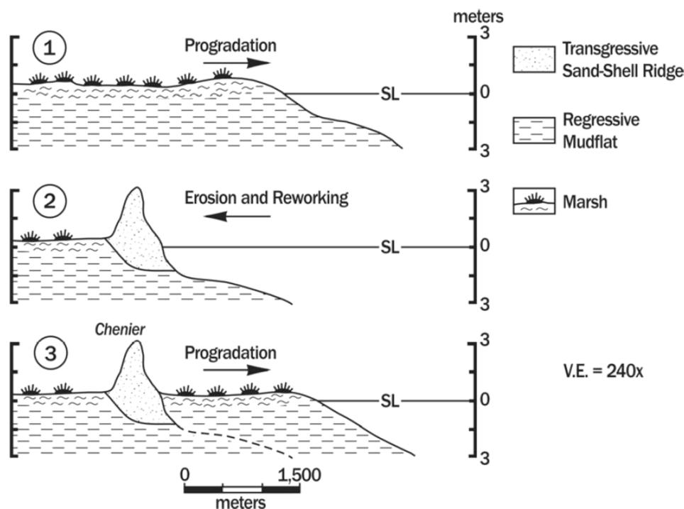
Fig. 2. Depositional model illustrating chenier plain development through mudflat progradation (1), wave erosion and reworking to create a transgressive ridge (2), and then mudflat progradation, which completes chenier genesis (3). SL = sea level [4].
