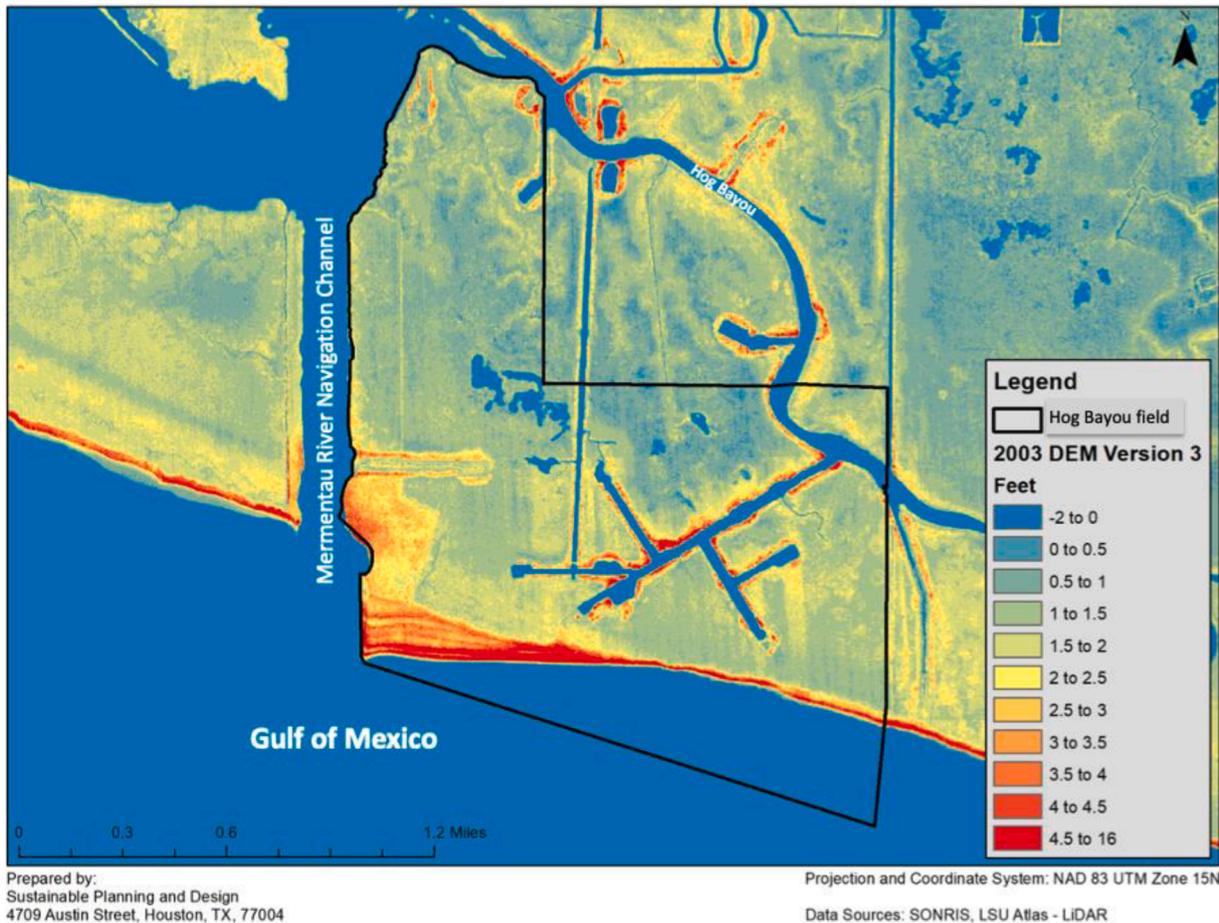
Fig. 18. Effect of navigation channel on Gulfward accretion of the beach-dune system east of the jetty. Elevations at the Hog Bayou area in 2003. The highest elevations are more than 1.2 m while the lowest elevations are at or below sea level. Note that ponds generally occur in wetlands with the lowest elevation.
