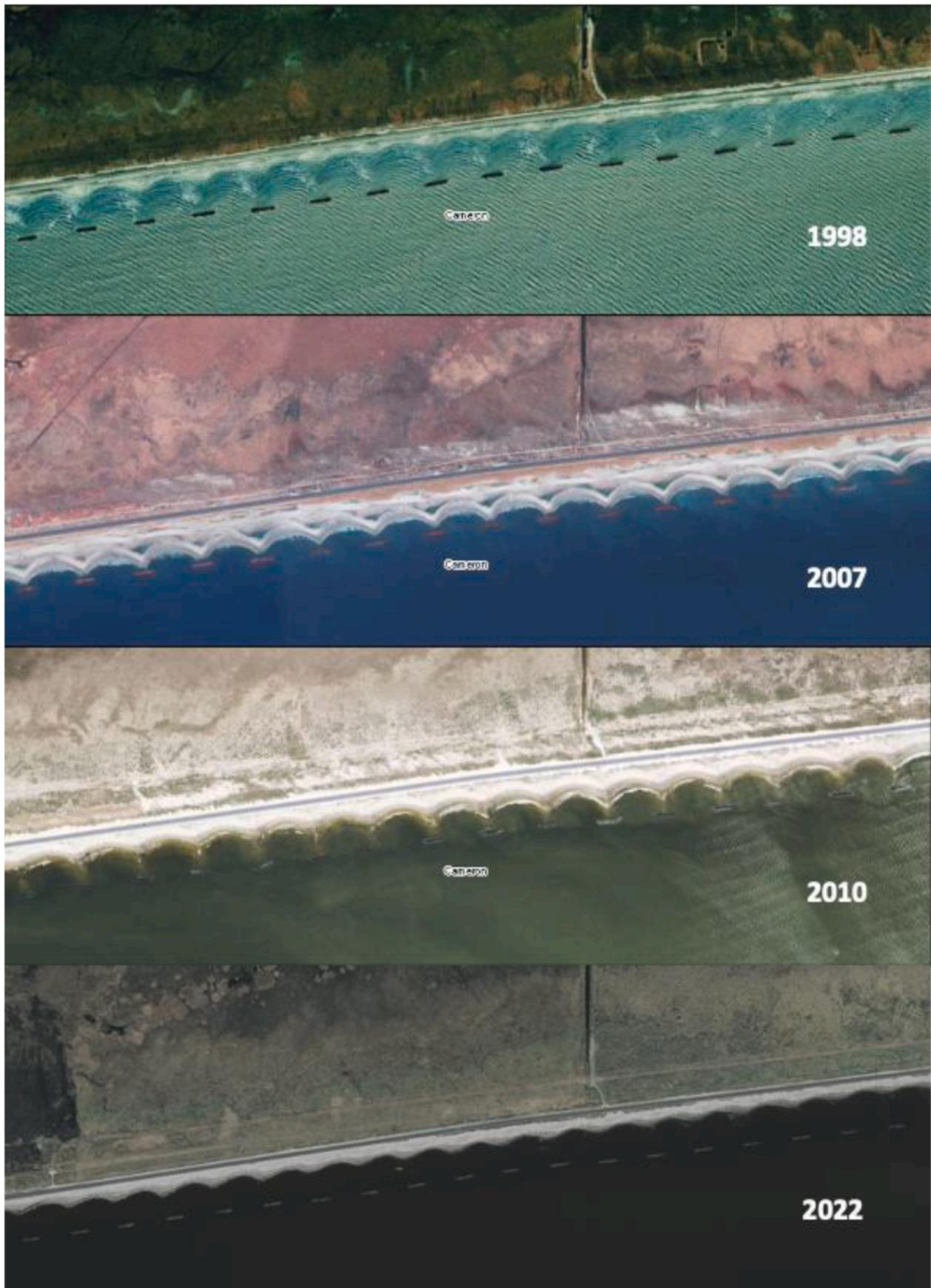
**Fig. 14.** Low-tide tombolos/high-tide salients at Holly Beach that formed as a result of the detached, segmented breakwaters [72]. Note that the 2022 image was taken after Hurricanes Laura and Delta (2020).
