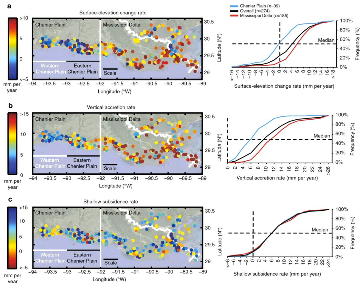
Fig. 8. Rates of surface elevation change (a), vertical accretion (b), and shallow subsidence (c) in coastal Louisiana [11].
