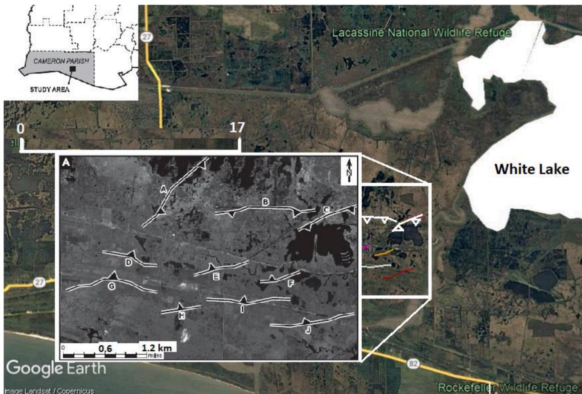
Fig. 5. Little Chenier area with detail inset showing active faults [62]. Tick marks are on the fault downtrown side. Note the presence of water bodies and their relationship to some of the faults.
