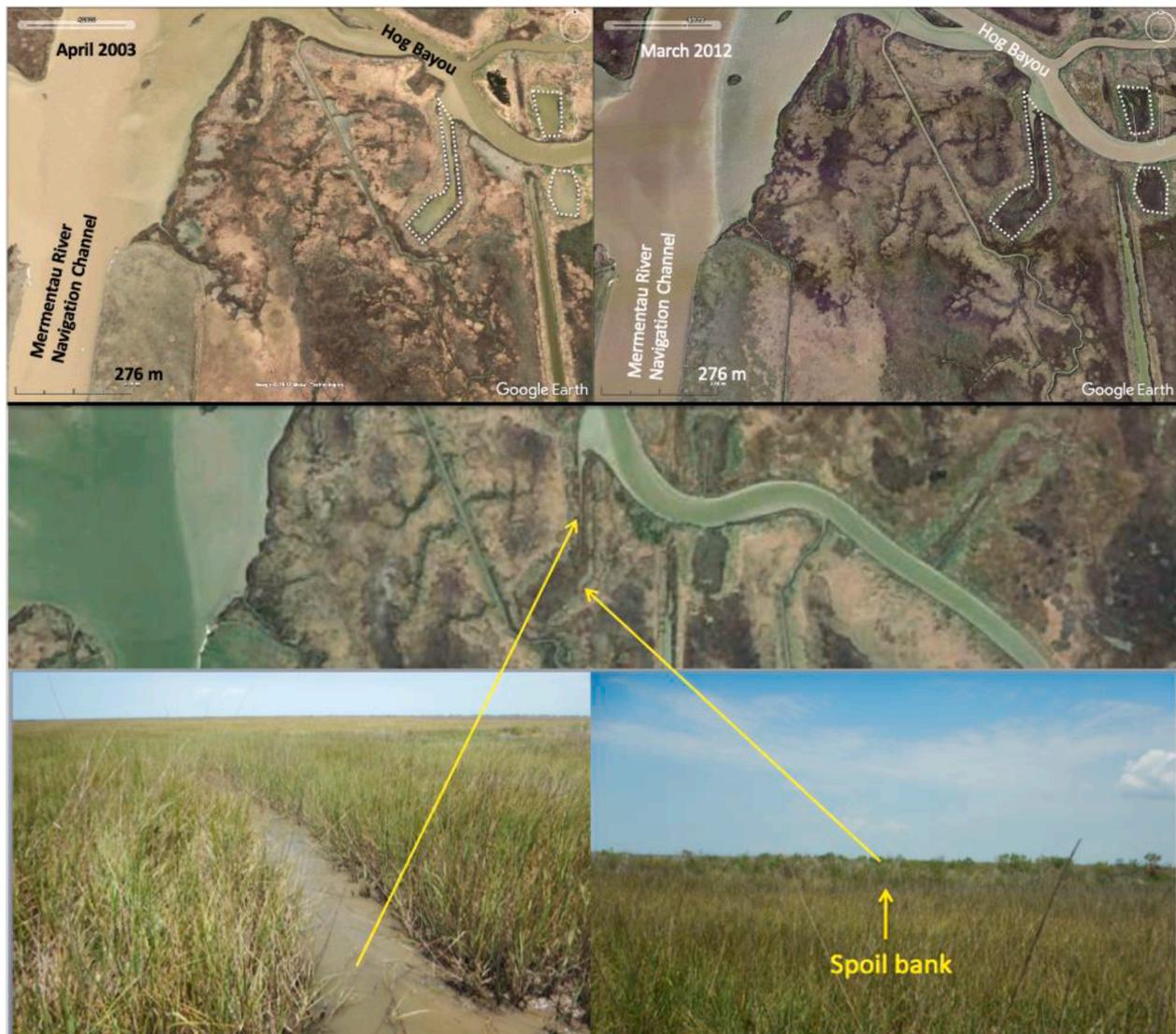
**Fig. 12.** Top: Infilling of a canal at the Hog Bayou oil and gas field (note outline). In 2003 the canal was unvegetated and by 2012 the canal has almost filled in with sediment (Google Earth). Bottom: The same canal has narrowed considerably and now supports marsh vegetation (Photos: Day and Hunter 2020). In 2020 the canal was less than 2 m in width although it had an initial width of about 30 m.
