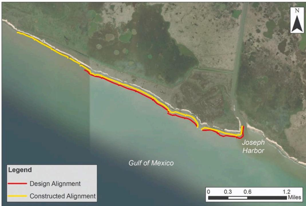
Fig. 16. Location of breakwater locations as designed (red) and as constructed (yellow)(HDR Engineering Inc.).
