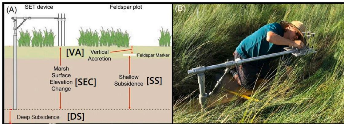
Fig. 4. (A) Measurements made at a CRMS station in the CPRA long-term marsh monitoring program focusing on how Surface Elevation Change (SEC) is determined using a Sediment Erosion Table (SET) modified from Jankowski et al. [11]. (B) Deploying a Sediment Erosion Table (SET) as described in Lane et al. (2020).
