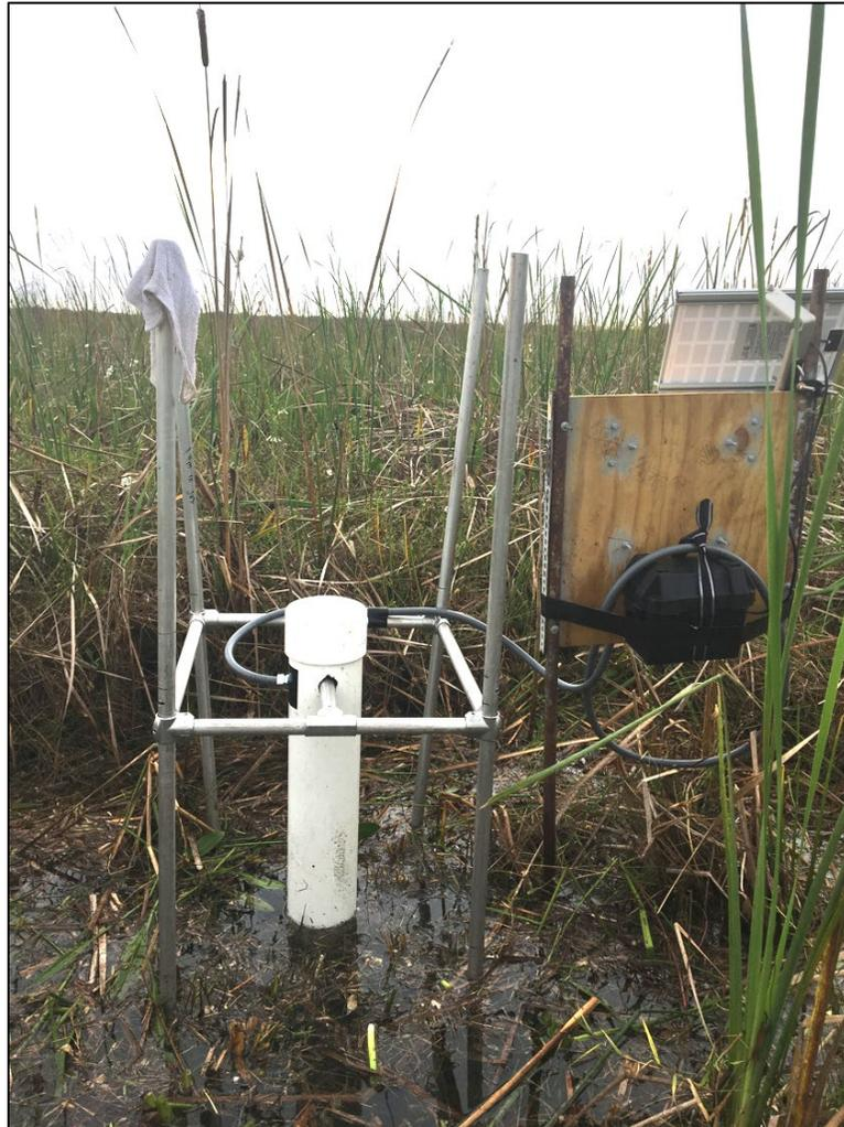
**Figure 12.** Photograph of the CR-SET deployment at the Fresh site (CRMS 3054) in November 2018.
