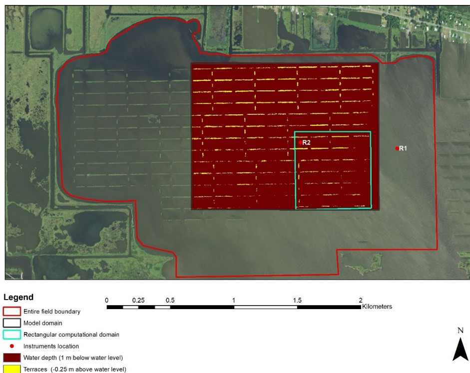
Figure 3.4 Rectangular terrace field of study showing the computational domain, bathymetry, and instruments location.
