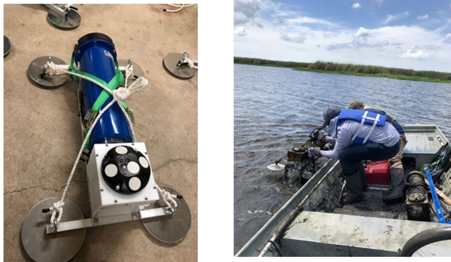
Figure 3.3 Nortek 1000 signature series ADCP mounted in aluminum frame (left). ADCP retrieval at a marsh terrace site in coastal LA. (right).
