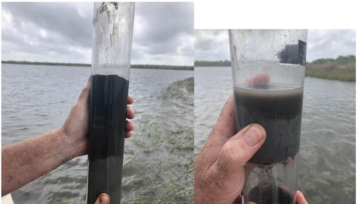
**Figure 32.** Piston cores from Yankee Canal subaqueous sites between the terraces, illustrating the visual differences between the interpreted pre-construction, stiff grey clay layer and the surficial black-brown and high porosity silt. Core YC8 (left) from an excavation pit shows a ~25 cm of distinct surficial material interpreted as post-construction deposition, while the deposit in core YC14 (right) on an adjacent (shallower) area that was not excavated is < 1 cm thick.
