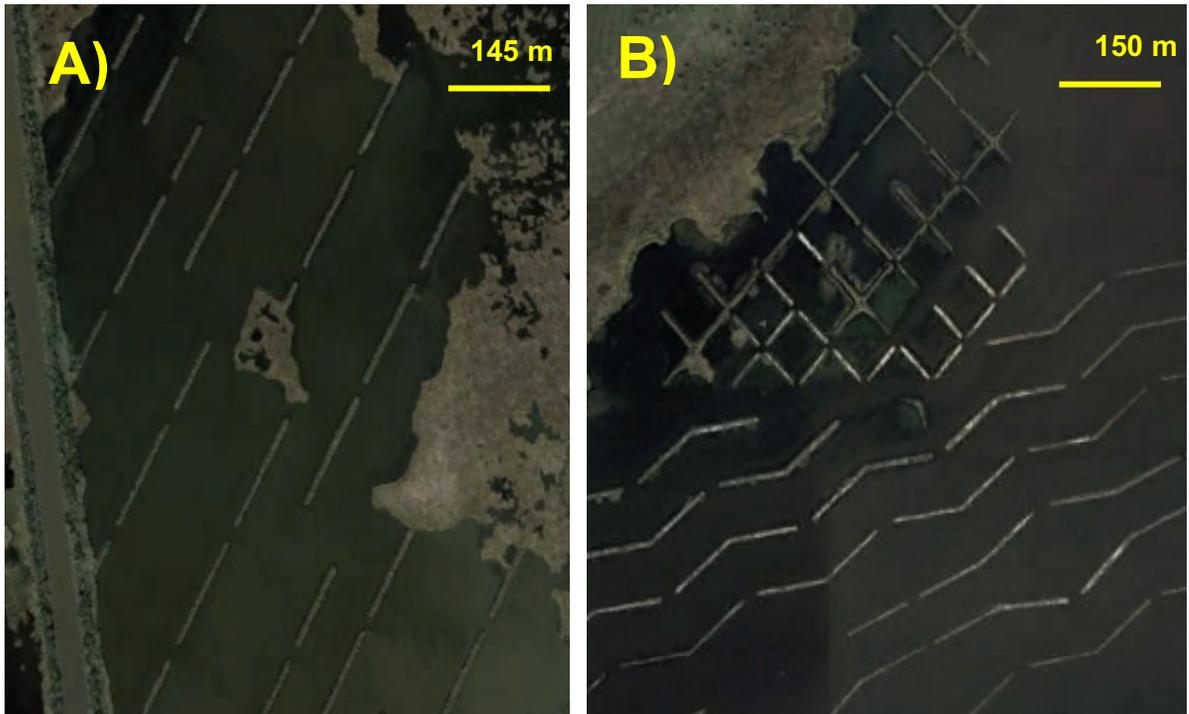
**Figure 5.** Google Earth satellite images of the three predominant marsh terraces designs (geometries) utilized in coastal Louisiana. Image (A) are linear terraces in Teal Pond, LA. Image (B) are grid terraces (top) and chevron (i.e., duck-wing) terraces (bottom) in Starks North Canal, LA.
