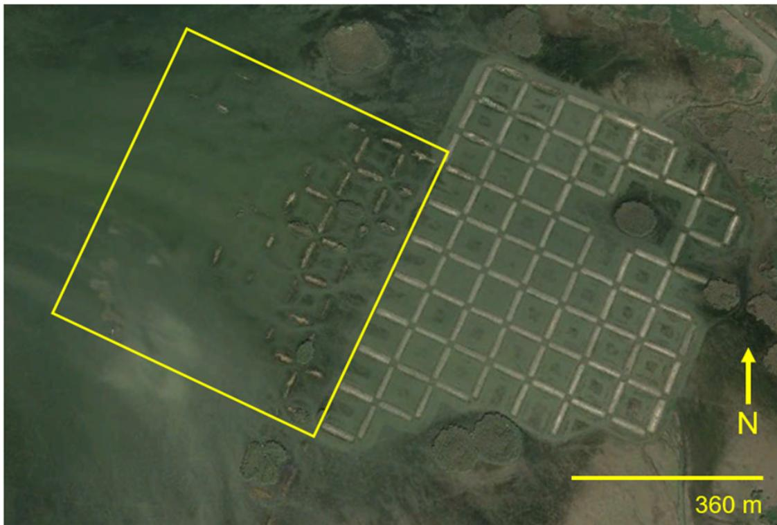
**Figure 12.** Google Earth 2019 satellite image of the Bay Alexis field study site. The degraded subaerial terraces shown on the left are remnants of the first terracing project in Bay Alexis completed in 2005, shortly before they were damaged by Hurricane Katrina. The more recent grid terrace field was constructed in 2015, which were funded by FEMA. The original extent of the 2005 field is illustrated by the yellow box.
