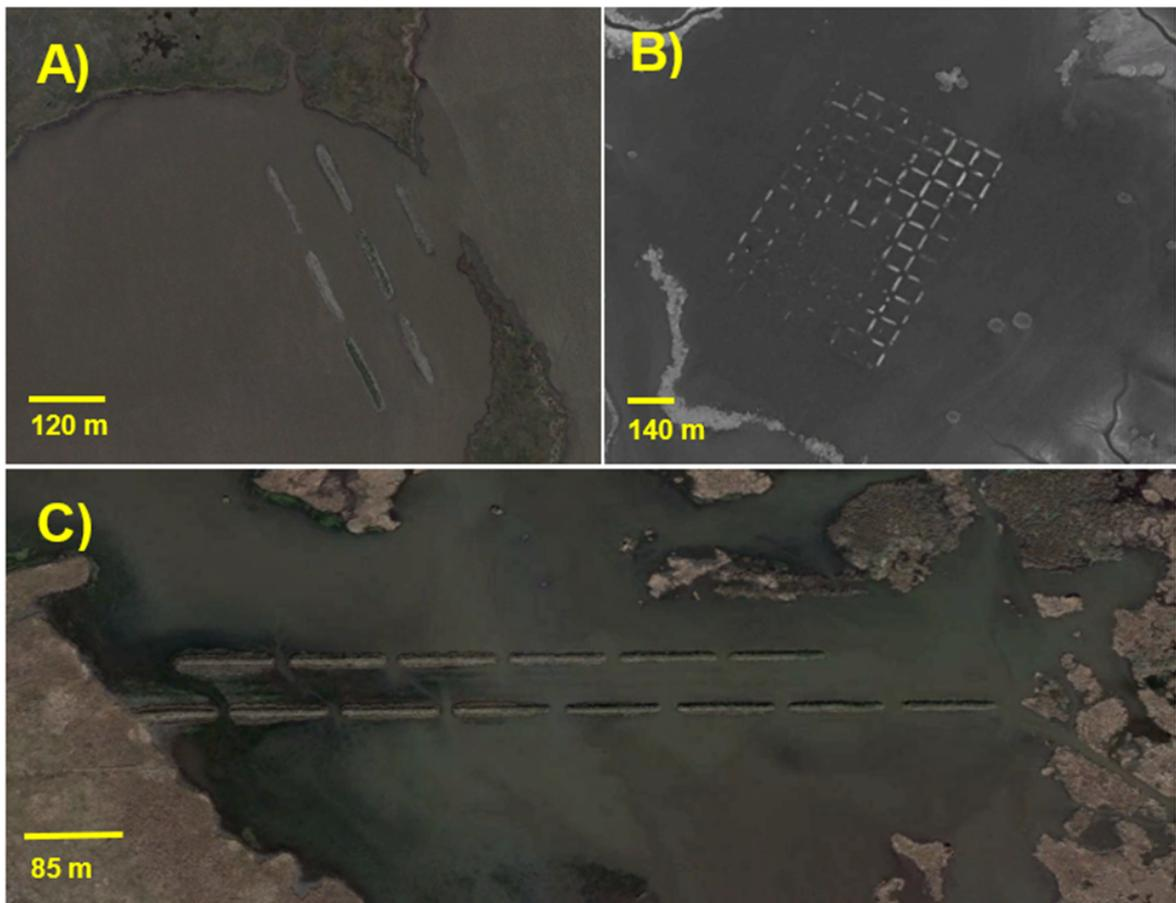
**Figure 7.** Google Earth satellite images of examples of the distribution of terraces in fields in projects carried out in coastal Louisiana. A) Linear terraces constructed in 2014 in Lake Tom on Marsh Island proximal to the shoreline and hydrological outlet of the lake. B) Grid terraces constructed in 2005 at Bay Alexis in the center of the bay. C) Linear terraces constructed in unnamed pond in 2015 south of Larose, LA that stretch across the entire water body.
