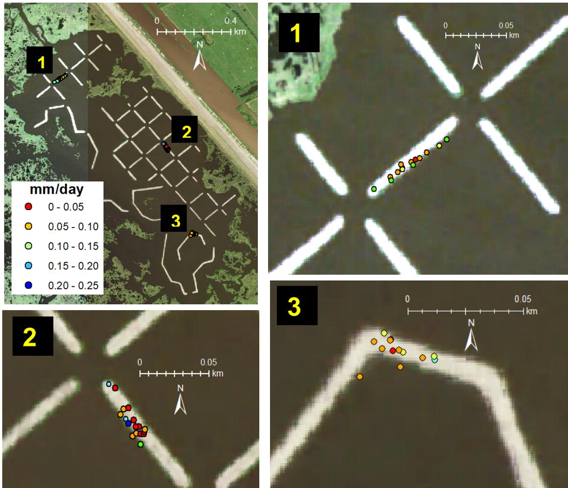
**Figure 22.** Deposition rates derived from feldspar plots at Bayou Monnaie over 71 days across 3 terraces. Values range from 0 mm/d to 0.25 mm/d (0 – 18 mm over 71 days). There is an inverse relationship between elevation and accretion on terraces at Bayou Monnaie.
