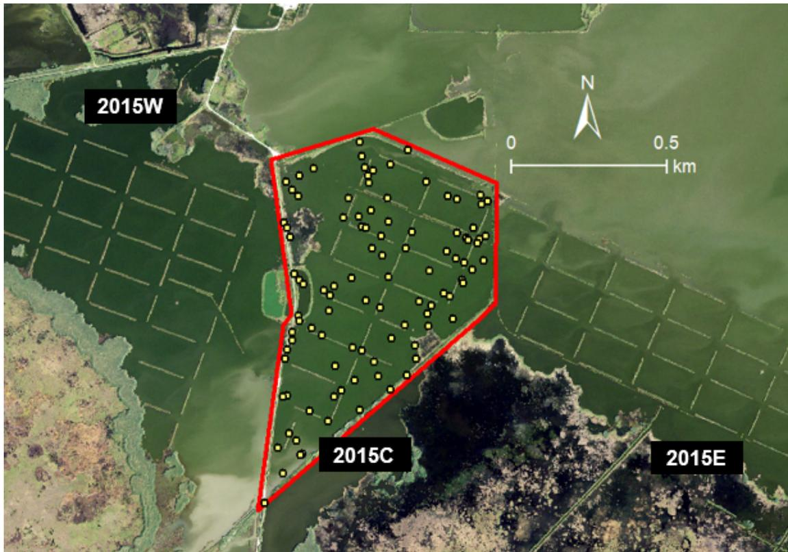
**Figure 18.** An example of the use of 102 accuracy assessment points (yellow circles) displayed on the terrace field at 2015C. Each site features 100 to 120 stratified random accuracy assessment points to compare classification results with ground-truth values derived from the NAIP true color imagery. Sites 2015W and 2015E are also labeled.
