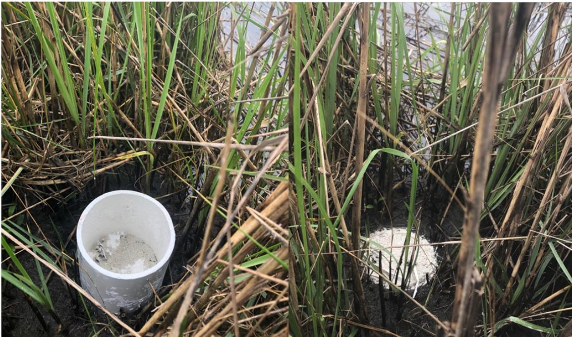
**Figure 15.** Feldspar marker horizon (FMH) plots. FMH plots were deployed on the subaerial portions of the terraces using a 10.8 cm diameter PVC ring laid on the terrace surface resulting in a thin layer (< 1 cm thick) plot with 183.85 cm<sup>2</sup> surface area.
