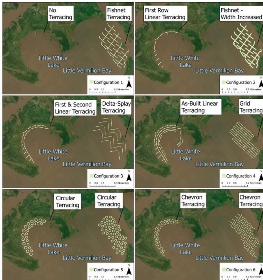
**Fig. 7. Model Configurations.** The figure conceptualizes the shapes of the terrace configurations for each of the six model simulations.
