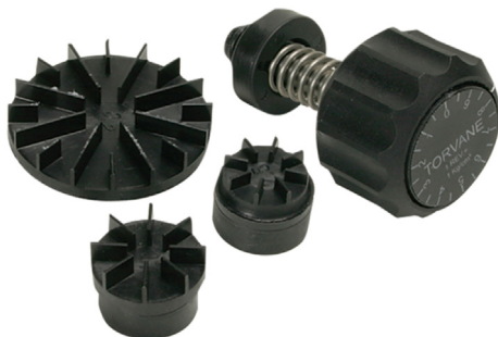
Fig. 15. Torvane with various diameter blades (photo courtesy of Humboldt).
