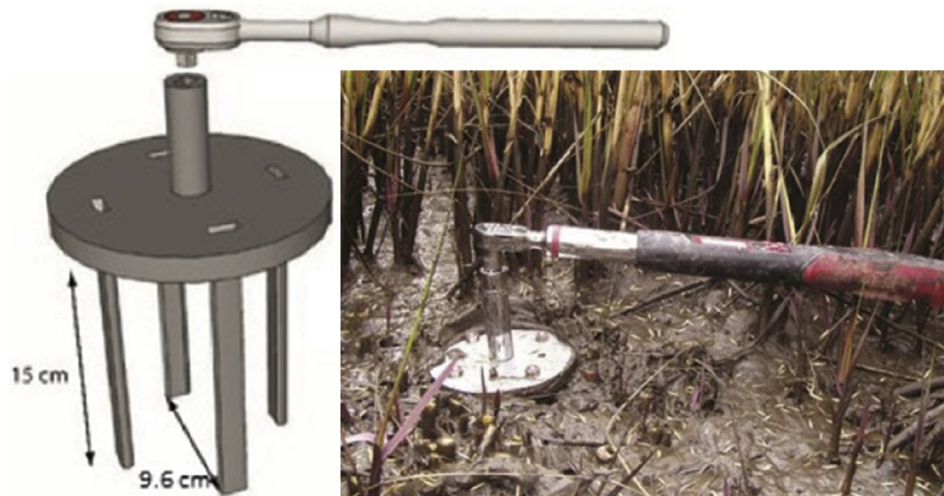
Fig. 20. Diagram and field use of the Wetland Soil Strength Tester (WSST) (modified from Sasser et al., 2018).
