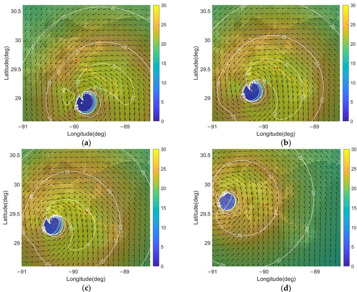
**Figure 3.** Distributions of hurricane winds (m/s) during Isaac (2012). White lines denote contour lines every 5 m/s. Black arrows denote wind direction. Two red symbols denote two levee-opening locations. (a) 03:00 UTC 29 August. (b) 08:00 UTC 29 August. (c) 11:00 UTC 29 August. (d) 17:00 UTC 29 August.
