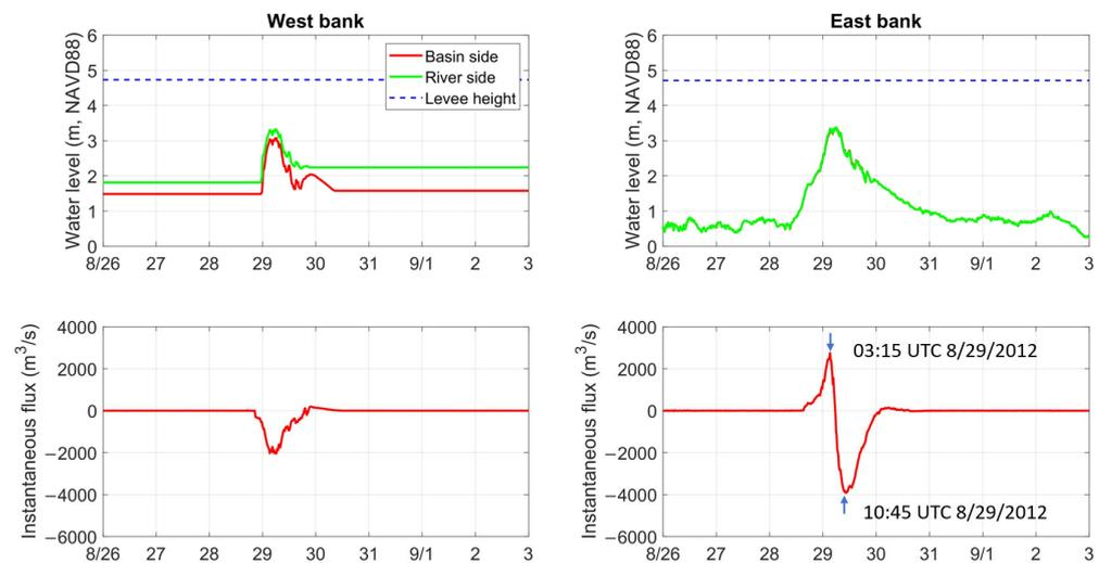
**Figure 7.** Time series of water level (m, NAVD88, top) and instantaneous flux ( $m^3/s$ , bottom) for west (left two) and east (right) banks at the upper-crossing location in the both-crossing case during Isaac (2012). The direction of positive flux is from west to east.
