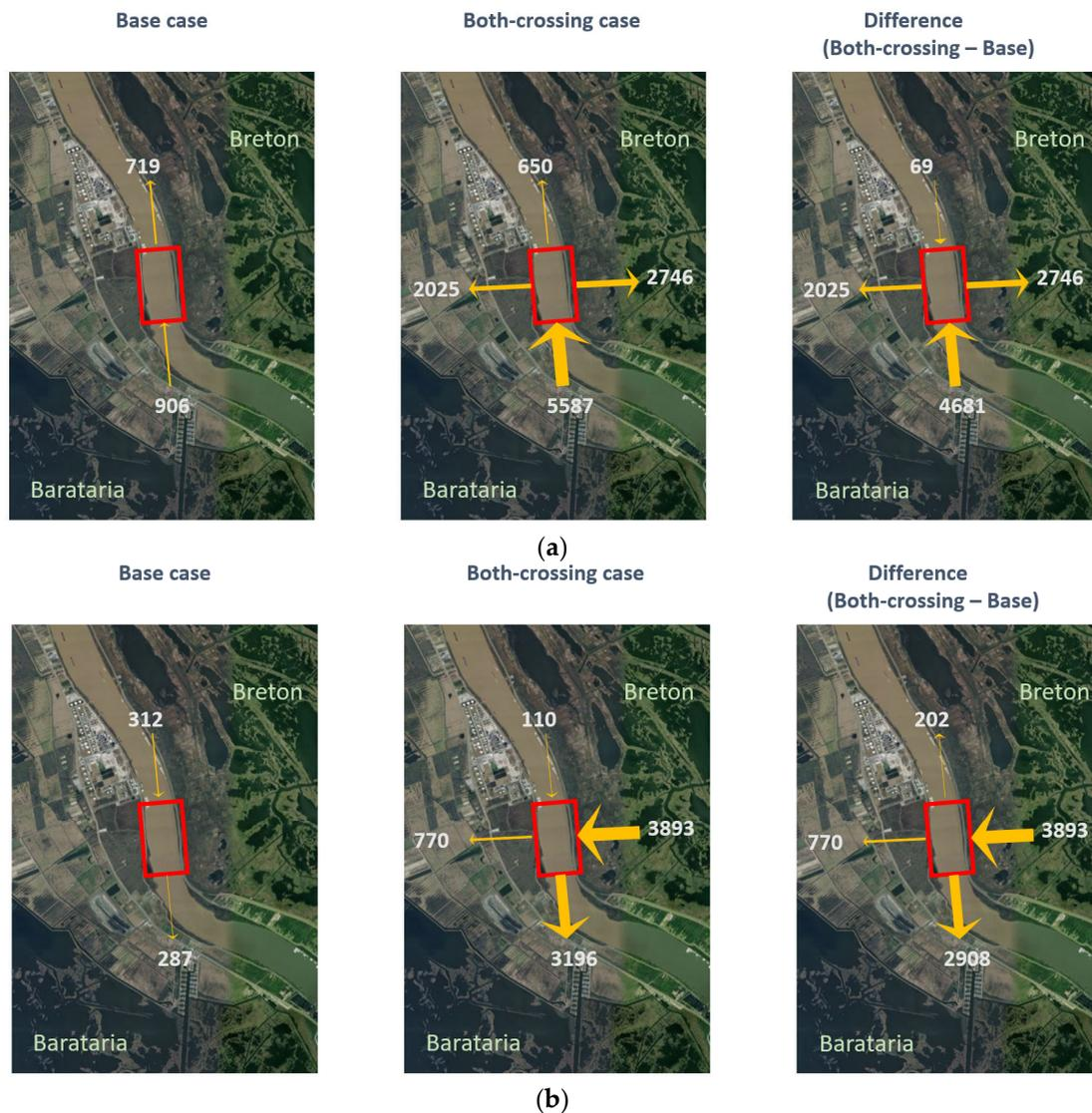
**Figure 8.** Flux ( $\text{m}^3/\text{s}$ ) analysis at the upper-crossing location for 03:15 UTC 29 August 2012 (top) and 10:45 UTC 29 August 2012 (bottom) during Isaac (2012). The thickness of flux arrow is proportional to the amount. (a) 03:15 UTC 29 August 2012. (b) 10:45 UTC 29 August 2012.
