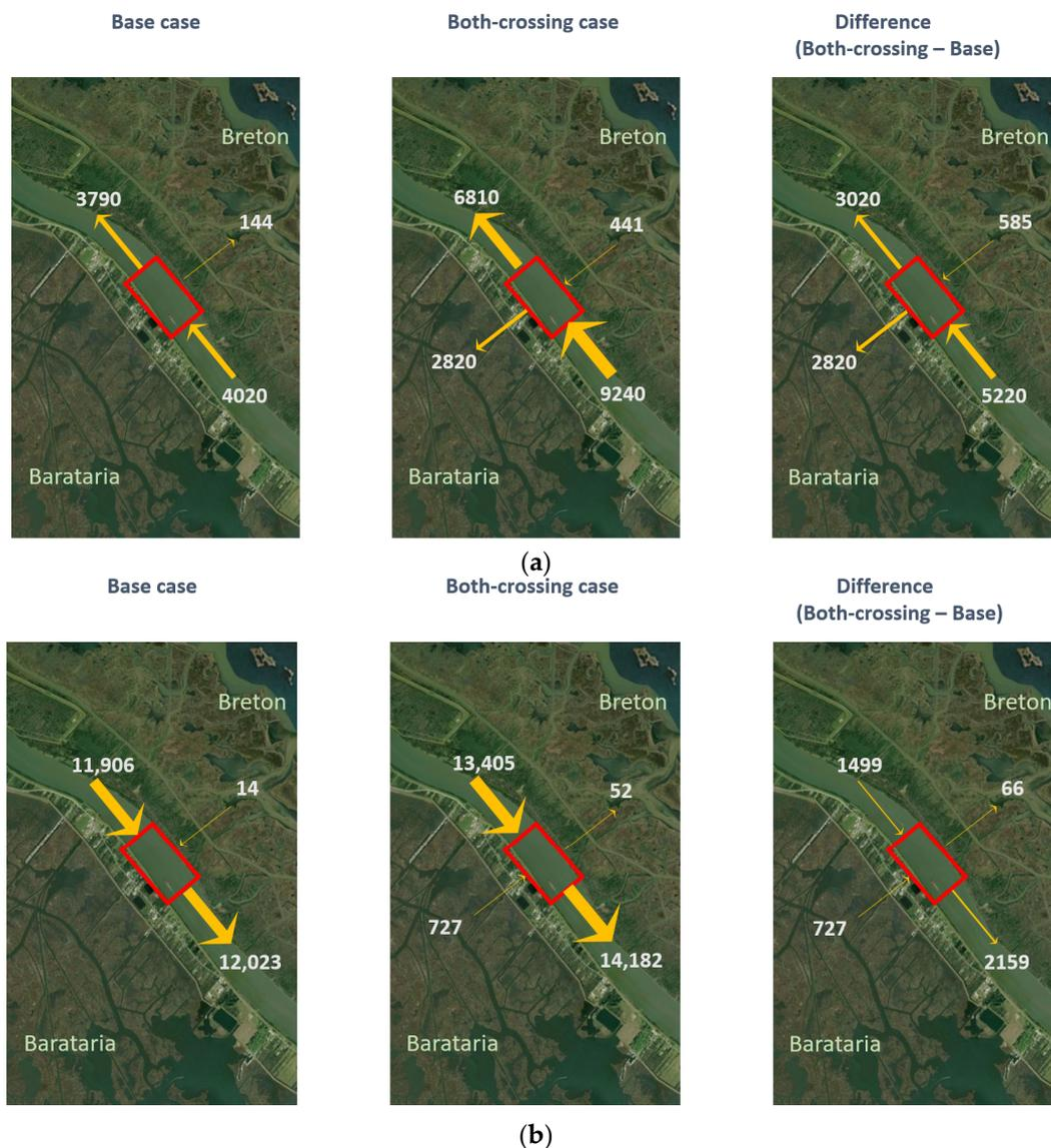
**Figure 11.** Flux (m<sup>3</sup>/s) analysis at the lower-crossing location for 02:45 UTC 8/29/2012 (top) and 16:45 UTC 8/29/2012 (bottom) during Isaac (2012). The thickness of flux arrow is proportional to the amount. (a) 02:45 UTC 29 August 2012. (b) 16:45 UTC 29 August 2012.
