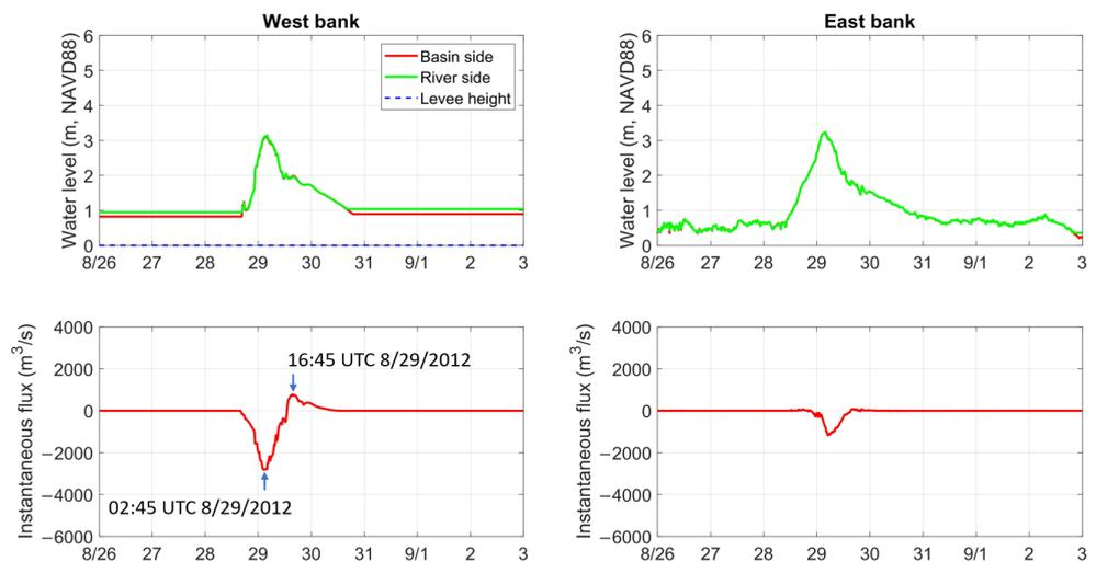
**Figure 10.** Time series of water level (m, NAVD88, top) and instantaneous flux (m<sup>3</sup>/s, bottom) for the west (left) and east (right) banks at the lower-crossing location in the both-crossing case during Isaac (2012). The direction of positive flux is from west to east.
