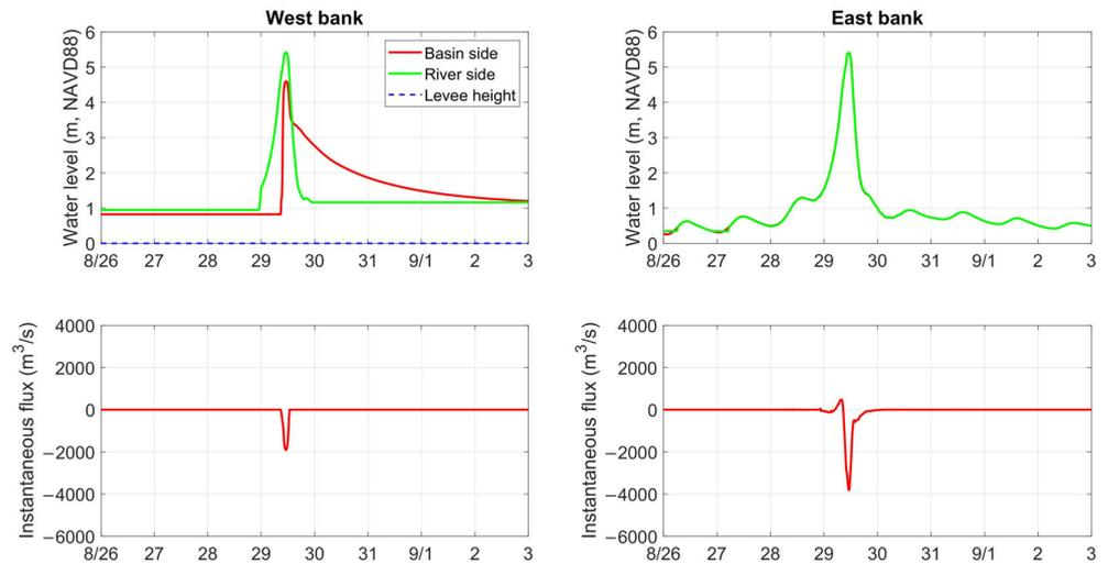
**Figure 9.** Time series of water level (m, NAVD88, top) and instantaneous flux (m<sup>3</sup>/s, bottom) for the west (left) and east (right) banks at the lower-crossing location in the base case during Isaac (2012). The direction of positive flux is from west to east.
