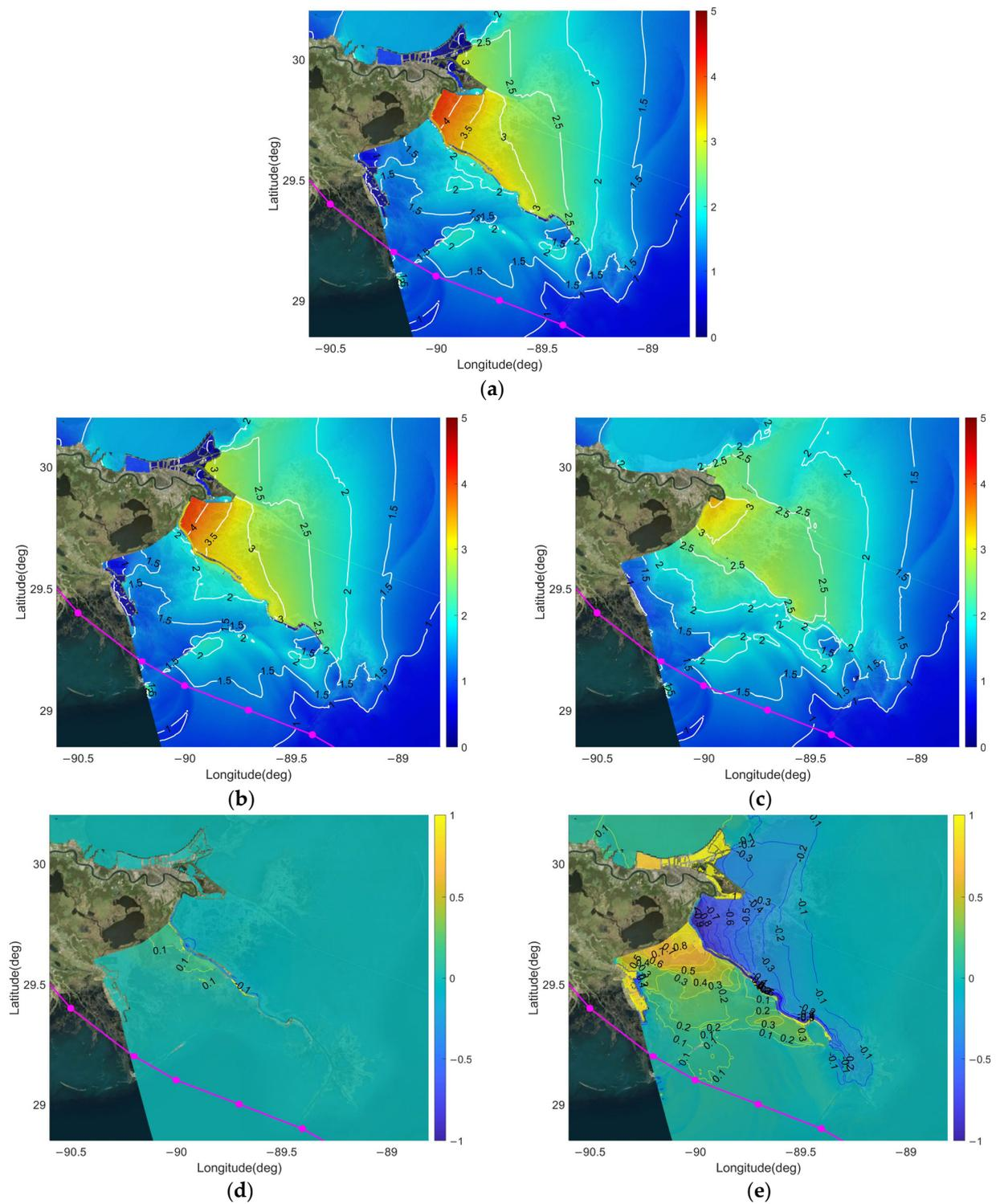
**Figure 5.** Maximum surge (m, NAVD88) and surge difference (m) distributions by Isaac (2012). (a) Base case (existing conditions); (b) Both-crossing case; (c) No-levée case; (d) Both-crossing case—Base case; (e) No-levée case—Base case. White lines denote contour lines every 1 m. Blue lines denote contour lines with negative values every 0.1 m. Yellow lines denote contour lines with positive values every 0.1 m. Magenta line with dots denotes the track of Isaac (2012).
