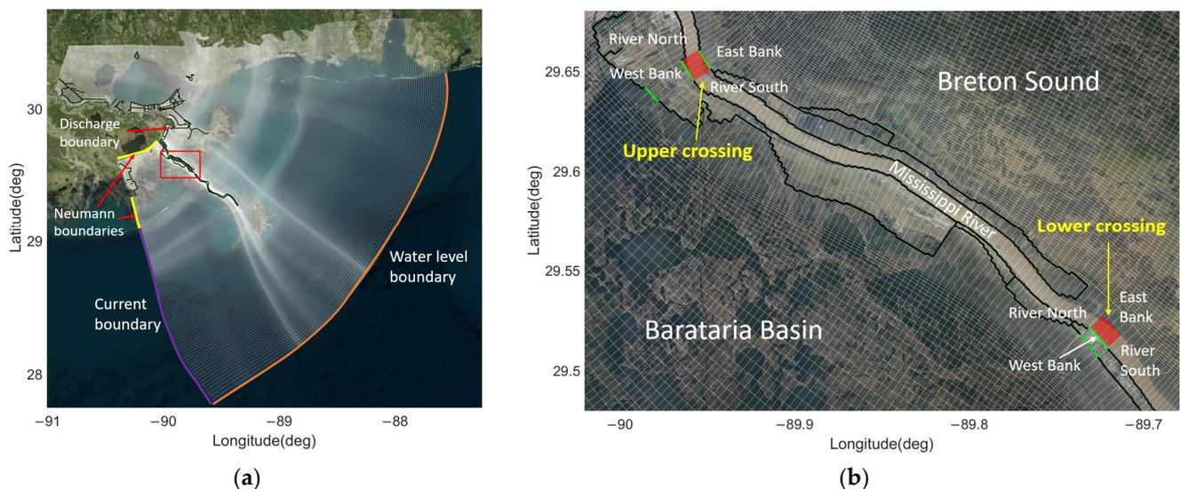
**Figure 2.** The model domain with computational grids (white line), boundaries (orange for water level, purple for current and yellow for Neumann) and the MR&T levee system (black line). Green lines denote the levee removal parts; filled red rectangles denote “control box” for flux analysis. (a) Entire model domain. (b) Local enlarged model domain.
