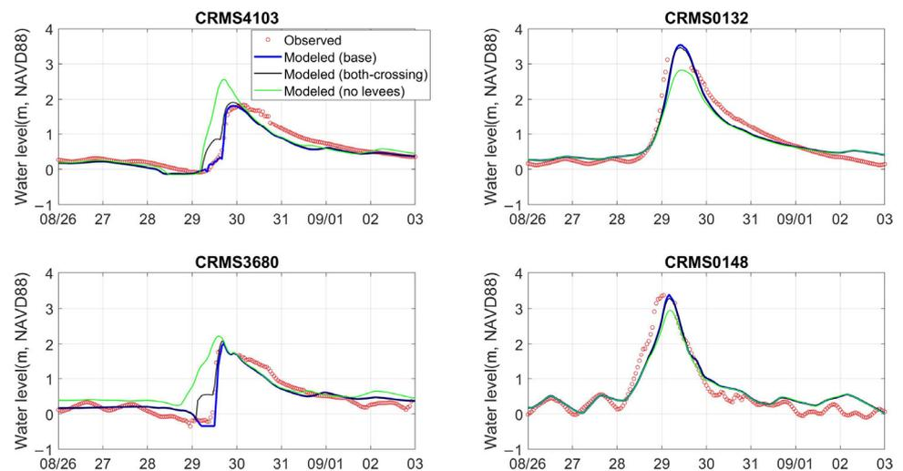
**Figure 4.** Comparisons of water level (m, NAVD88) time series between the observed (red circle) and the modeled phenomena in three scenarios (blue line for the base case, black line for the both-crossing case and green line for the no-levee case) at four CRMS stations during Hurricane Isaac (2012).
