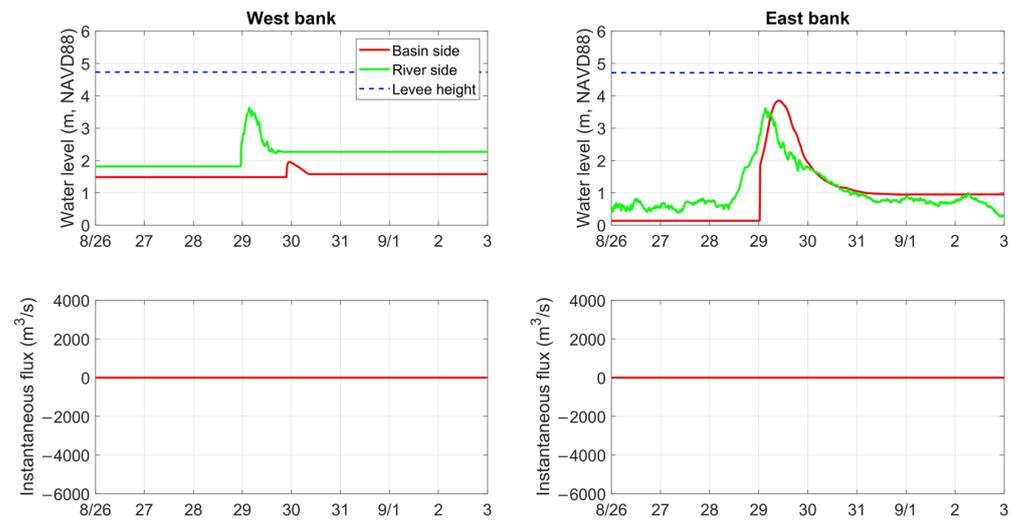
**Figure 6.** Time series of water level (m, NAVD88, top) and instantaneous flux ( $m^3/s$ , bottom) for the west (left) and east (right) banks at the upper-crossing location in the base case during Isaac (2012). The direction of positive flux is from west to east.
