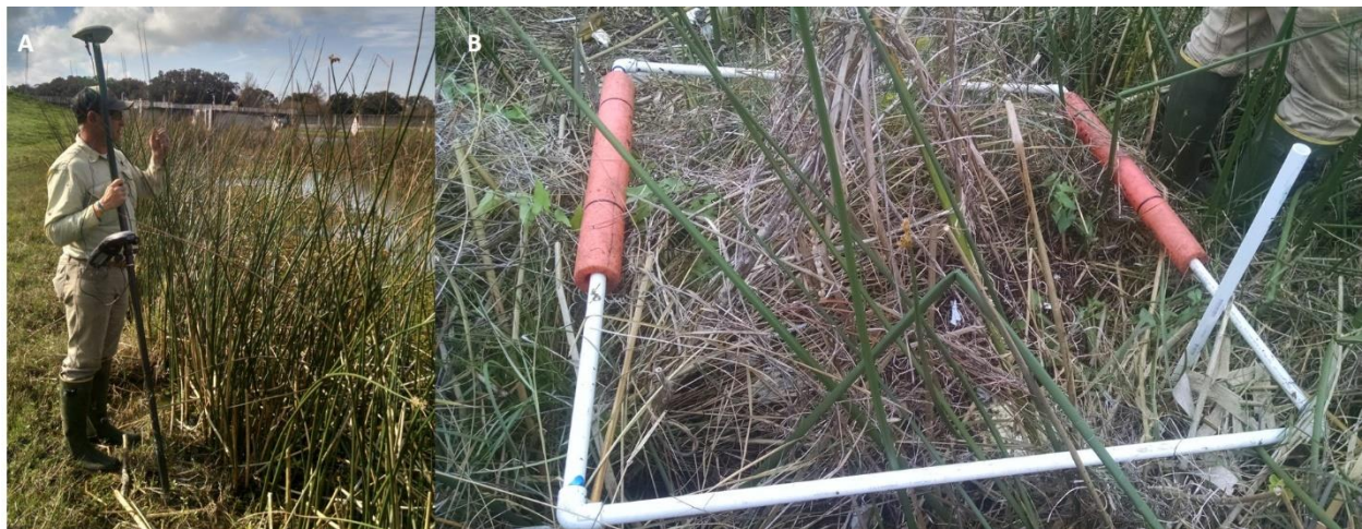
Figure 2 Elevation measurements were taken using a Geo Explorer 6000 GeoXR GPS attached to a Zephyr Model 2 GNSS receiver (A); vegetation was surveyed using a modified Braun-Blanquet 1-meter squared method (B)
