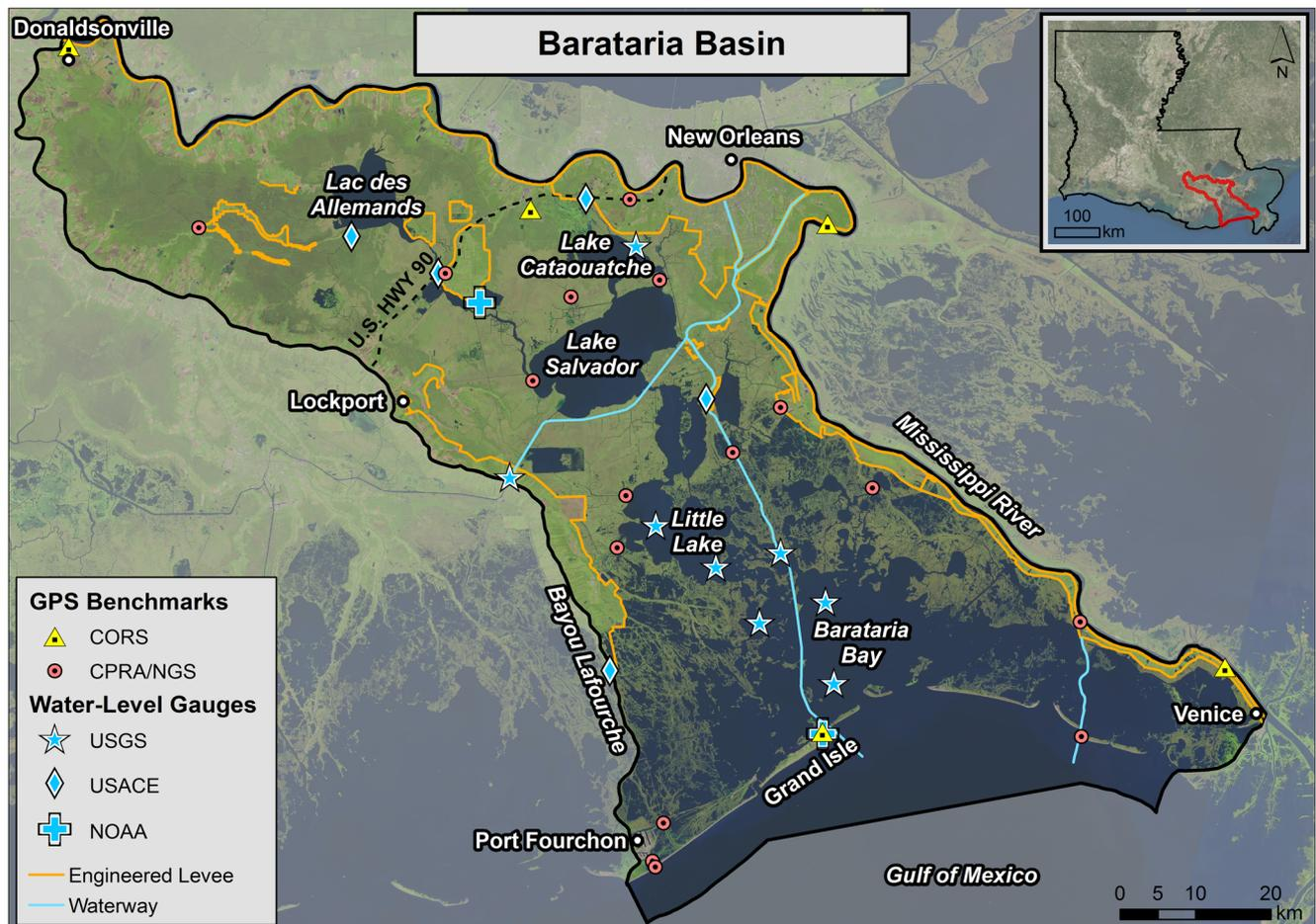
**Fig. 2** Satellite image (Landsat 8 OLI/TIRS) illustrating the hydrologic boundary and physiographic features for the Barataria Basin, as well as GPS benchmark and water-level gauge locations for evaluating subsidence
