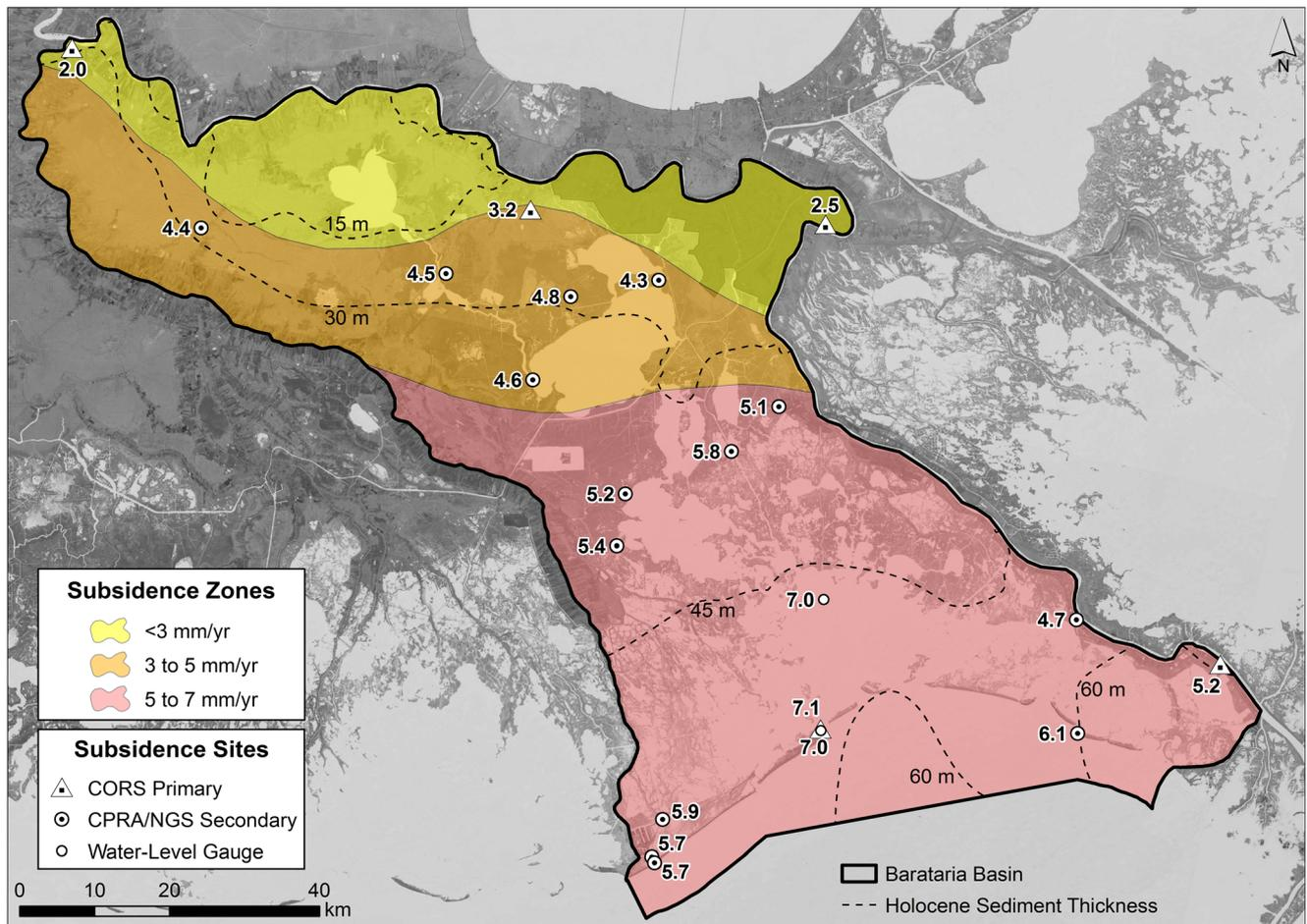
**Fig. 7** Subsidence zones identified for Barataria Basin based on high-resolution elevation change measurements at benchmarks and water-level gauges. Holocene sediment thickness contours illustrate a general
